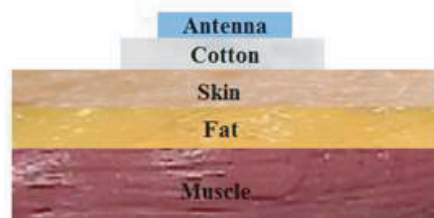
Figure 1. Layered model of human tissue with antenna.
