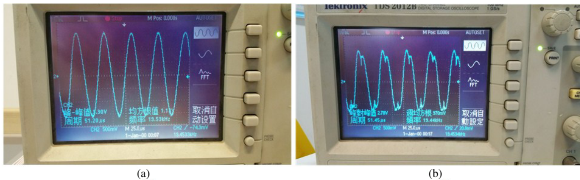
Figure 8. Measured voltage waveforms of Honeywell sensor: (a) right above the power track ( X : 25 \mu\text{s}/\text{div} , Y : 500 \text{ mV}/\text{div} ); (b) right above the gap ( X : 25 \mu\text{s}/\text{div} , Y : 500 \text{ mV}/\text{div} ).
