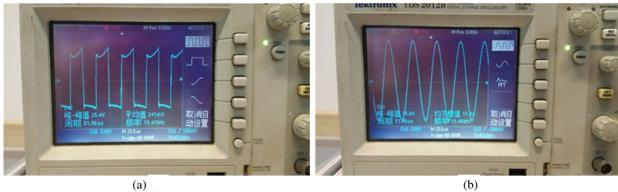
Figure 7. Measured voltage waveforms: (a) power track ( X : 25 \mu\text{s}/\text{div} , Y : 5 \text{ V}/\text{div} ); (b) pickup coil ( X : 25 \mu\text{s}/\text{div} , Y : 5 \text{ V}/\text{div} ).
