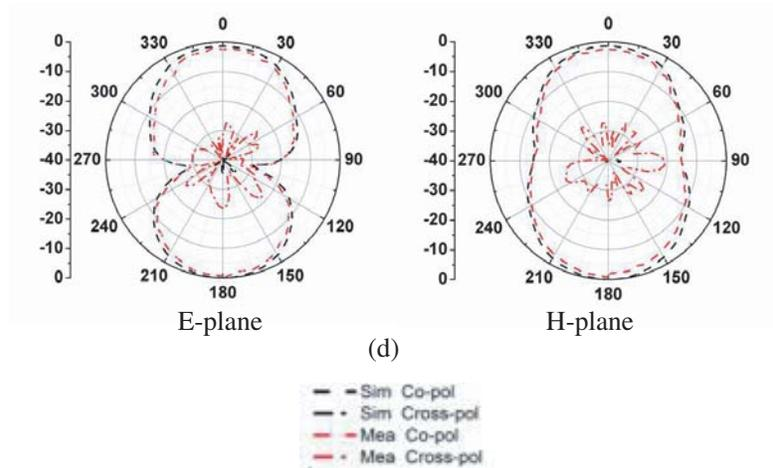
**Figure 5.** 2-D radiation pattern of the proposed antenna: (a) 3.1 GHz; (b) 4.5 GHz; (c) 7.1 GHz; and (d) 9.5 GHz.
