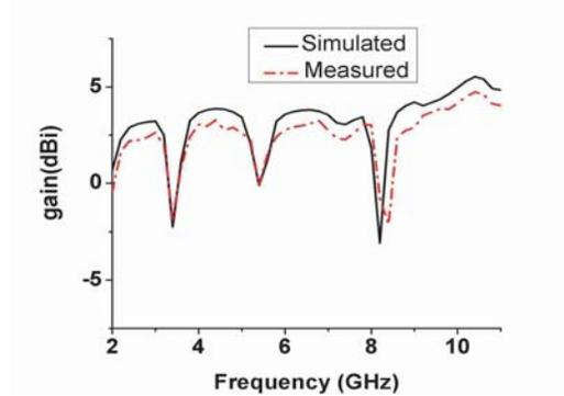
**Figure 6.** Simulated and measured gains of the proposed antenna.
