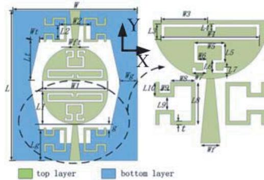
**Figure 1.** Topology of the proposed antenna.
