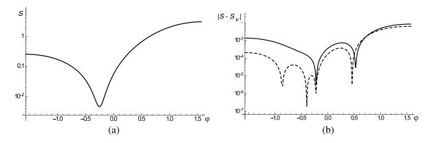
Figure 8. (a) The scattering intensity as calculated from the contrast current. (b) The absolute difference between the scattering intensity S and validation data  $S_V$ , the solid line is with the contrast current from the simulation, the dashed line is with the contrast current from the exact solution, represented by the same discretization as the simulation.
