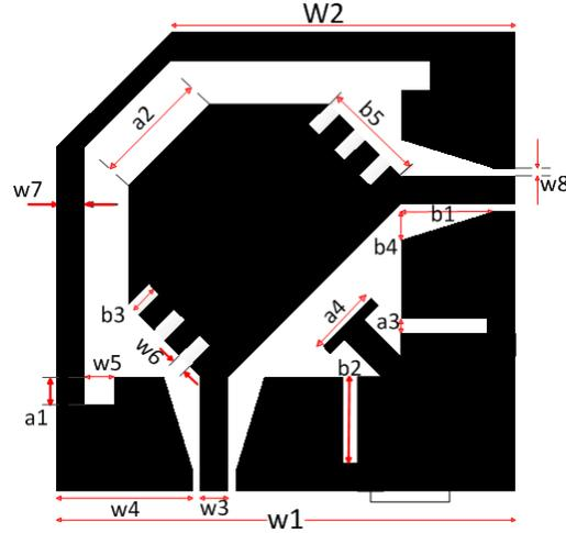
**Figure 1.** Geometry of CPW-fed MIMO antenna.
