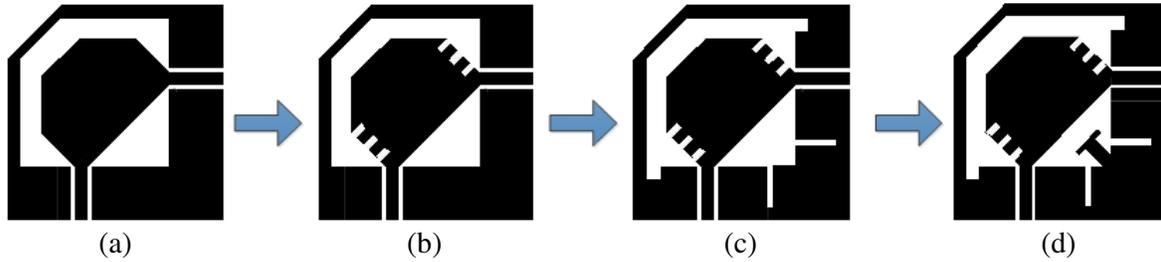
**Figure 2.** The process of this antenna design.
