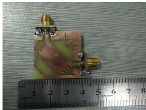
**Figure 4.** Photograph of the CPW-fed MIMO antenna.
