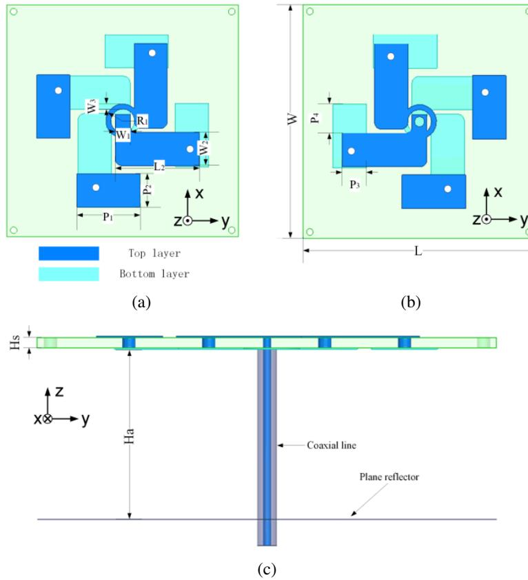
**Figure 1.** Geometry of the proposed antenna. (a) Top view. (b) Bottom view. (c) Side view with a plane reflector.
