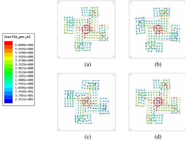
**Figure 4.** The simulated current distribution on the crossed dipoles at 2.5 GHz for (a)  $0^\circ$ , (b)  $90^\circ$ , (c)  $180^\circ$ , (d)  $270^\circ$ .
