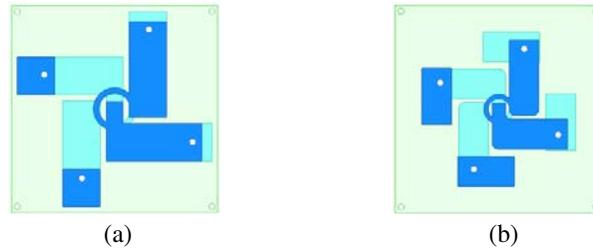
**Figure 2.** The process of antenna design. (a) Square radiating patches, (b) improved model.
