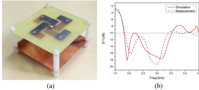
**Figure 5.** A prototype and the reflection coefficients of the fabricated antenna.
