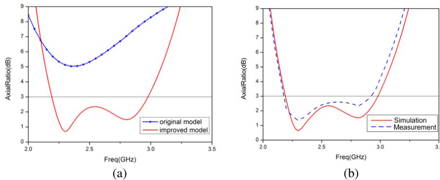
**Figure 3.** (a) Simulated axial ratio for original and improved model. (b) Measured and simulated axial ratio.
