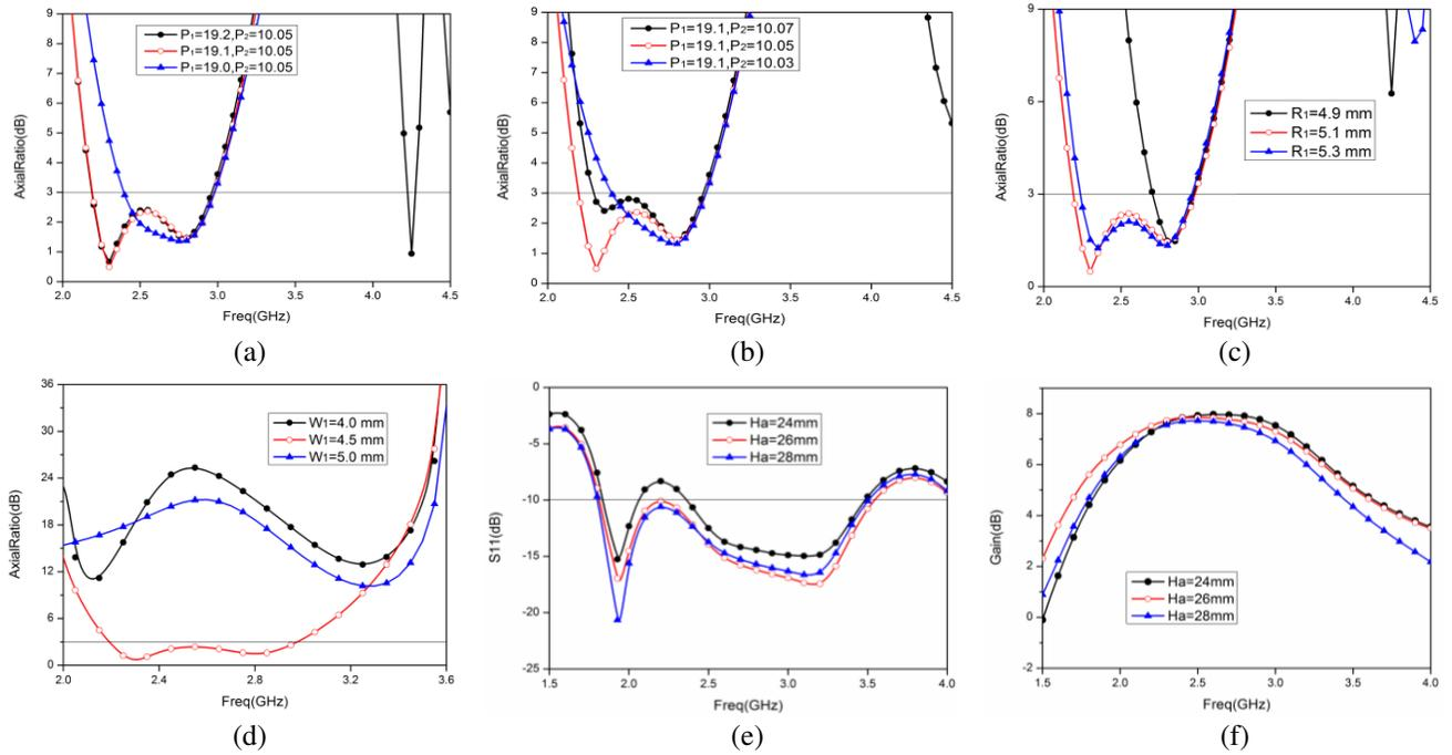
**Figure 6.** (a) Simulated axial ratio for different  $P_1$ . (b) Simulated axial ratio for different  $P_2$ . (c) Simulated axial ratio for different  $R_1$ . (d) Simulated axial ratio for different  $W_1$ . (e) Simulated reflection coefficients for different  $Ha$ . (f) Simulated RHCP gain for different  $Ha$ .
