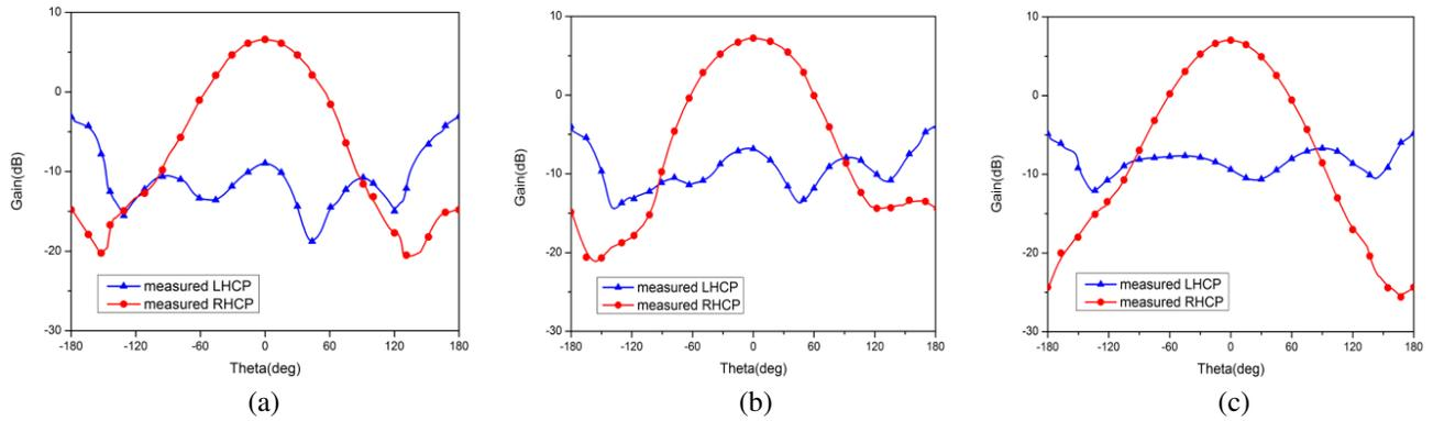
**Figure 7.** Radiation patterns of the antenna at (a) 2.2 GHz, (b) 2.5 GHz, (c) 2.9 GHz.
