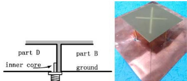
**Figure 2.** Feed structure and prototype of proposed antenna.
