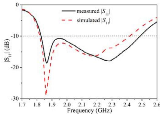
Figure 8. Simulated and measured  $|S_{11}|$  of proposed antenna.
