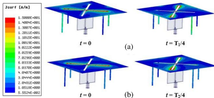
Figure 5. Current distribution of the proposed antenna at (a) 2.04 GHz and (b) 2.34 GHz.
