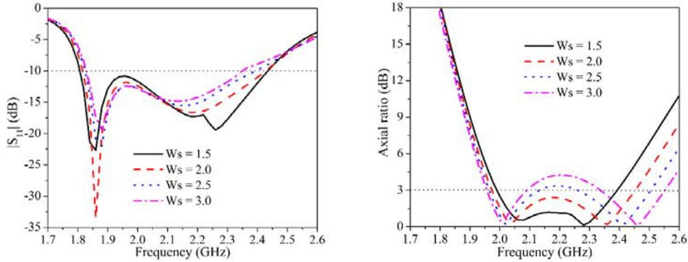
**Figure 6.** Simulated  $|S_{11}|$  and AR of the proposed antenna for different  $W_s$ s.
