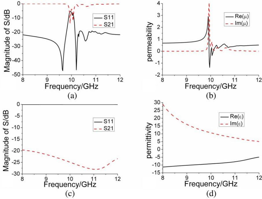
**Figure 2.**  $S$  parameters and the real part and imaginary part of the retrieved effective electromagnetic parameters, (a) magnitude of  $S$  for ferrite-only case, (b) effective permeability for ferrite-only case, (c) magnitude of  $S$  for rods-only case, (d) effective permittivity for rods-only case.
