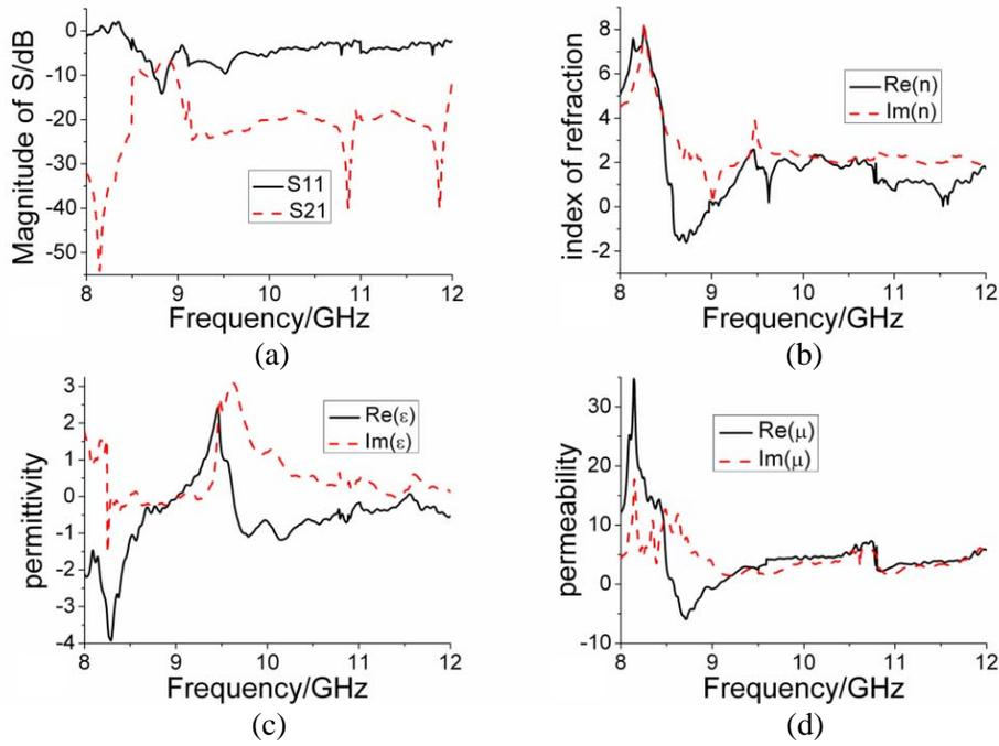
**Figure 8.** Experimental  $S$  parameters and the real part and imaginary part of the retrieved effective electromagnetic parameters for ferrite-dielectric metamaterial at  $H = 3400$  Oe. (a) Magnitude of  $S$ , (b) index of refraction, (c) effective permittivity, and (d) effective permeability.
