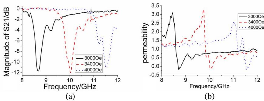
**Figure 7.** (a) Experimental transmission parameters  $S_{21}$ , (b) the real part and imaginary part of the effective permeability for ferrite-only case under different bias magnetic fields.
