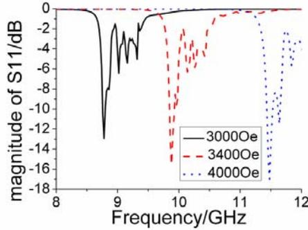
**Figure 4.** Transmission parameters  $S_{11}$  of the metamaterial under different bias magnetic fields.
