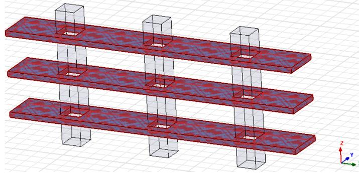
**Figure 1.** Anisotropic metamaterial model consists of ferrite and rods. The incident electromagnetic wave is transmitted along the Y direction. The magnetic field is in the X direction and the electric field is in the Z direction, the bias magnetic field is along Z direction. The ferrite sheets are  $22.86 \times 3 \times 0.4 \text{ mm}^3$  and the rods are  $1.5 \times 1.5 \times 10.16 \text{ mm}^3$ , respectively.
