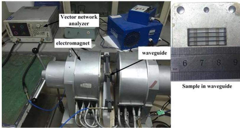
**Figure 5.** Experimental waveguide setup, the sample is placed between the air gap of the electromagnet. The bias magnetic field is tuned by adjusting the input current.
