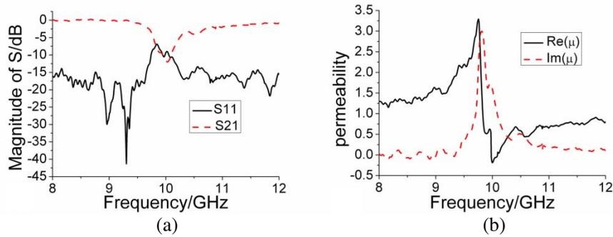
**Figure 6.** (a) Experimental  $S$  parameters, (b) the real part and imaginary part of the effective permeability for ferrite-only case at  $H = 3400$  Oe.
