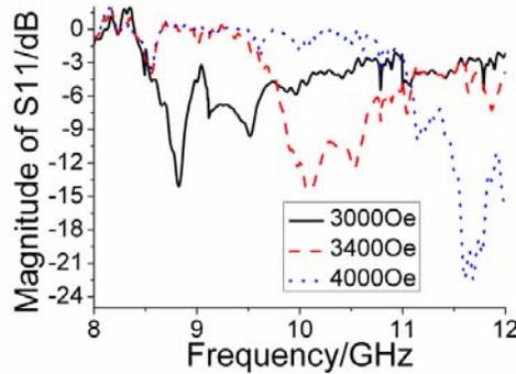
**Figure 9.** Experimental transmission parameters  $S_{11}$  of the metamaterial under different bias magnetic fields.
