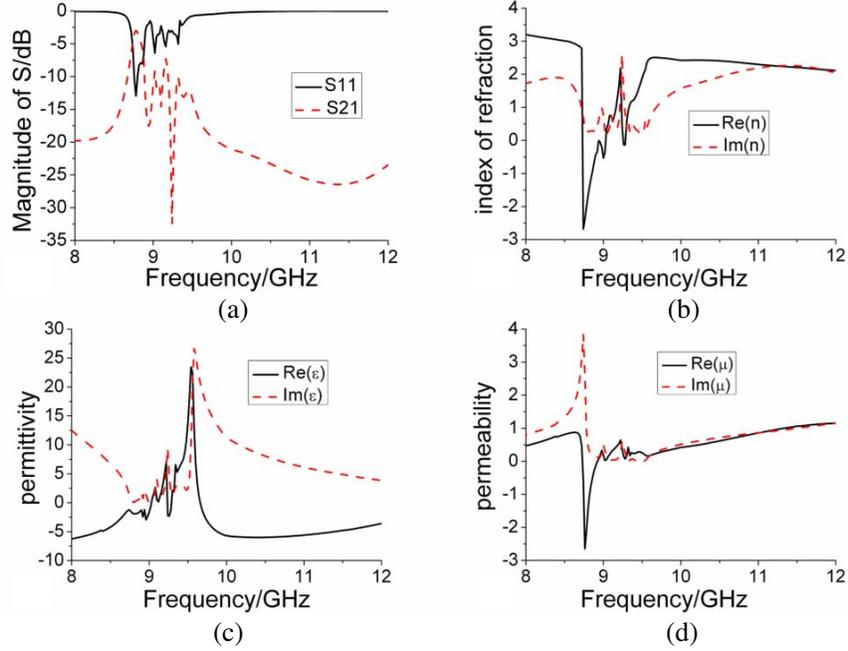
**Figure 3.**  $S$  parameters and the real part and imaginary part of the retrieved effective electromagnetic parameters for ferrite-dielectric metamaterial at  $H = 3000$  Oe, (a) magnitude of  $S$ , (b) index of refraction, (c) effective permittivity, (d) effective permeability.
