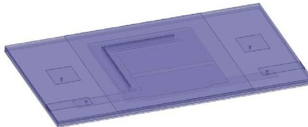
**Figure 5.** The whole view of the DFQMSIW filter.
