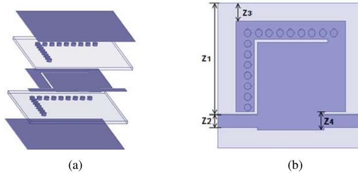
**Figure 1.** (a) The structure of DFQMSIW resonator; (b) Top view of DFQMSIW resonator.
