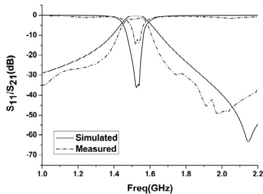
**Figure 7.** The simulated and measured results of the two-order DFQMSIW filter.
