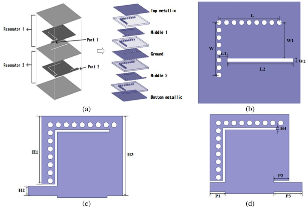
**Figure 4.** The structure of the DFQMSIW filter: (a) The topology structure of the DFQMSIW filter cavities; (b) The top view of Ground; (c) The top view of Middle 1; (d) The top view of Middle 2.
