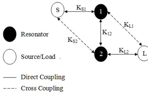
**Figure 3.** Coupling scheme of the proposed two-cavity filter.
