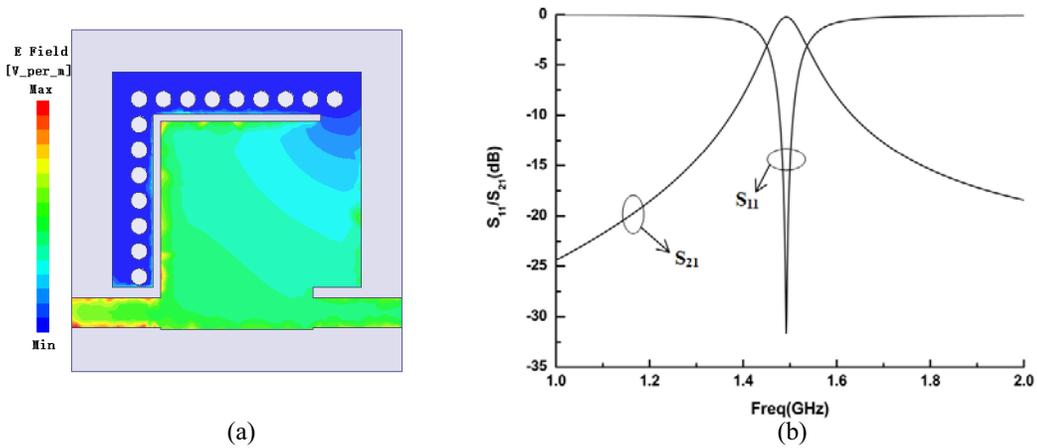
**Figure 2.** (a) Magnitude of electric field distribution in the cavity at resonator frequency; (b) Frequency response of the DFQMSIW resonator.
