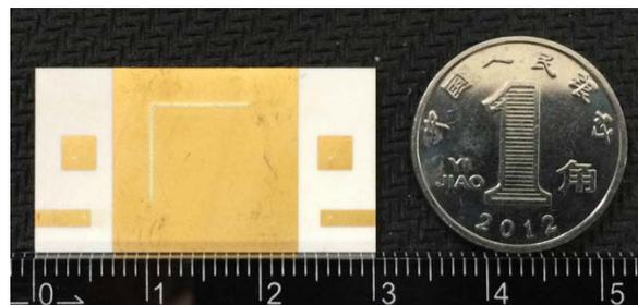
**Figure 6.** The picture of the two-order DFQMSIW filter.
