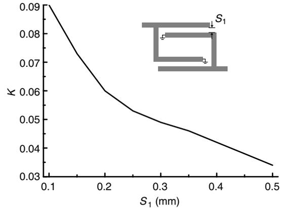
**Figure 3.** Variation of  $k$  against the coupling gap ( $s_1$ ) of the open/shorted coupled lines.
