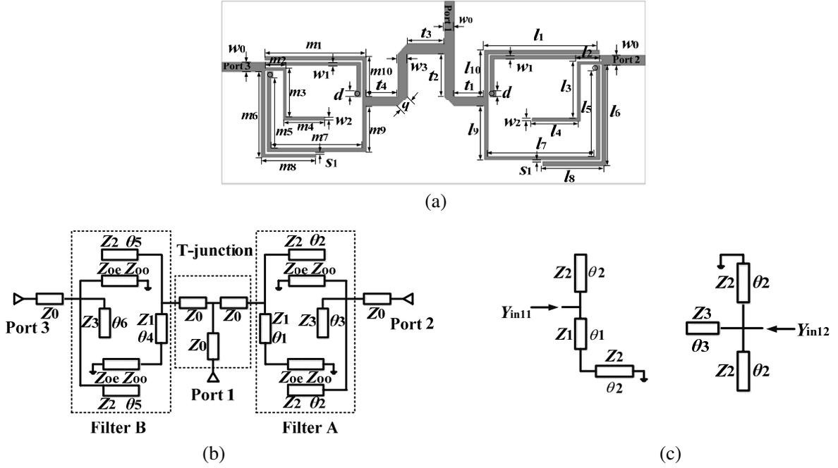
**Figure 1.** Structure and circuits of proposed microstrip diplexer. (a) Top view of the diplexer, (b) equivalent circuit of the diplexer, (c) the input admittance  $Y_{in}$  of the filter A.
