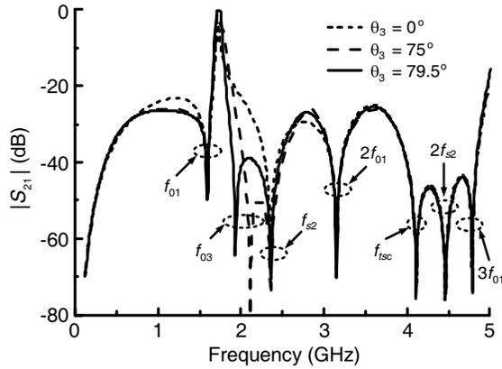
**Figure 2.** Simulated frequency responses versus  $\theta_3$  of the filter A,  $\theta_1 = 66^\circ$ ,  $\theta_2 = 102^\circ$ .
