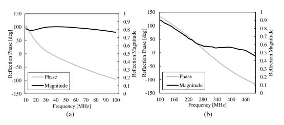
Figure 4. Reflection phase shift and magnitude for (a) AMC 1 and (b) AMC 2.
