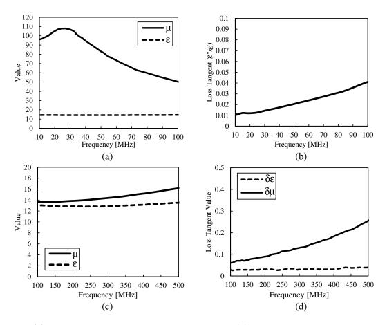
Figure 2. (a) Permeability and permittivity values; (b) and dielectric loss tangent for the  $Ni_{0.8}Cu_{0.1}Zn_{0.05}Co_{0.05}Fe_{1.92}O_4$  in the VHF range. (c) Permeability and permittivity values; (d) and dielectric loss tangent  $(Ba_{0.5}Sr_{0.5})_3Co_2Fe_{24}O_{41} + 0.2wt.\%$  WO<sub>3</sub> in the VHF/UHF range. All parameters were extracted from the results presented in [8].
