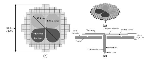
**Figure 3.** (a) Perspective view of antenna system; (b) top view of the antenna system with critical dimensions. (c) Side-view showing the feeding mechanism used to excite the radiator. Standard 50-ohm coax are used for the feed without a balun. Note that only one set of poles is shown here, similar scheme is used for the orthogonal poles as well.
