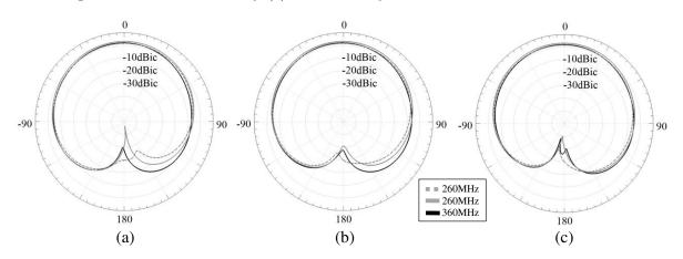
**Figure 6.** Simulated radiation patterns of the RHCP gain for the above frequencies at (a)  $\phi = 0^{\circ}$ , (b)  $\phi = 45^{\circ}$ , and (c)  $\phi = 90^{\circ}$ , legend of frequencies shown below applies to all plots.
