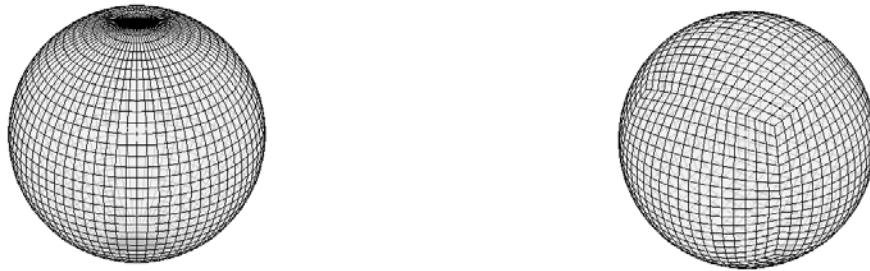
Figure 3. Examples of grids obtained with the two sampling schemes with an equatorial angular resolution of 0.2 samples per degree. The Conventional sampling scheme with 2664 samples is to the left and the Cubed Sphere sampling scheme with 1946 samples is to the right.
