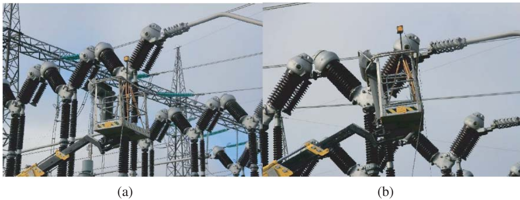
Figure 6. Arrangements for further measurements with the probe at (a) 6.83 m and (b) 7.63 m.
