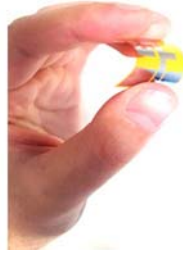
Figure 1. Flexible inkjet printed monopole antenna based on a Kapton Polyimide substrate.
