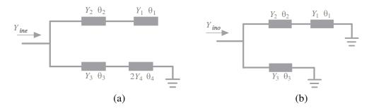
**Figure 3.** The Equivalent circuit model of the proposed square ring multiple-mode resonator. (a) Even mode circuit model. (b) Odd mode circuit model.
