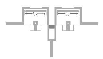
Figure 7. Layout of the proposed UWB power divider with notched band.
