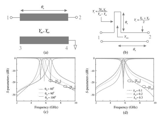
Figure 5. (a) Schematic of the parallel coupled lines. (b) Equivalent circuit of the parallel coupled lines. (c) Effect of the electrical length  $\theta_n$  at  $f_n = 5.8$  GHz on the central frequency of the notched band ( $k_n = 0.2$  fixed). (d) Effect of the coupling coefficient  $k_n$  on the bandwidth of the notched band ( $\theta_n = 90^\circ$  at  $f_n = 5.8$  GHz fixed).
