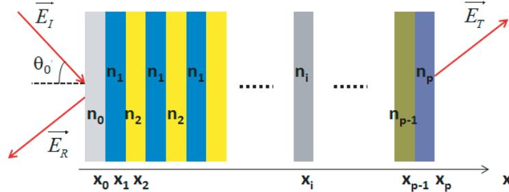
**Figure 1.** Propagation of light through a multilayer structure consisting of the two different materials with different indices of refraction.
