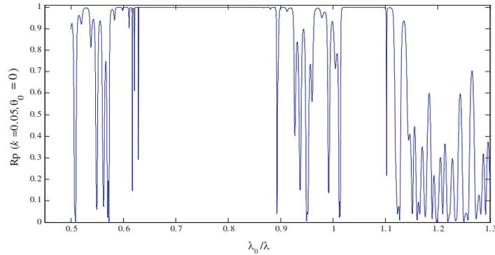
**Figure 9.** Reflection response of the deformed  $Bg_{27}/Ag_4/Bg_{27}$  system at normal incidence and for  $k = 0.05$ .
