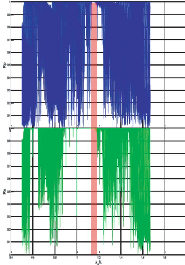
**Figure 6.** The reflection response for  $TE$  and  $TM$  polarizations according to the normalized wavelength.
