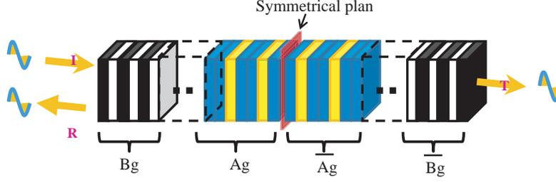
**Figure 2.** An example of a hybrid symmetrical quasi-periodic system having the form  $Bg_n/Ag_m/Bg_n$ .
