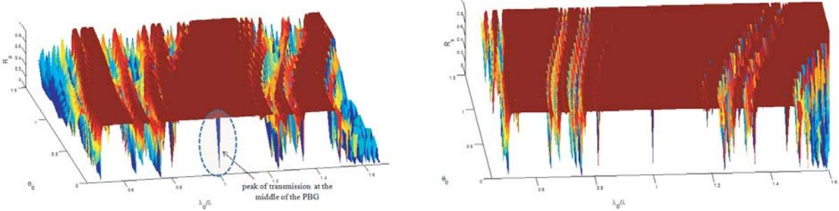
**Figure 3.** Variation of the reflection spectrum according to the normalized wavelength  $\frac{\lambda_0}{\lambda}$  and the incidence angle  $\theta_0$  for both polarization  $TE$  and  $TM$ .
