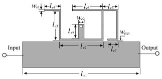
Figure 2. Geometry of proposed triple-mode SLR.
