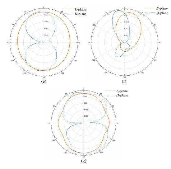
**Figure 4.** Measured radiation pattern of the UWB planar monopole antenna: (a) 2.5 GHz, (b) 3.0 GHz, (c) 5.0 GHz, (d) 5.2 GHz, (e) 7.5 GHz, (f) 8.0 GHz, (g) 10.0 GHz.
