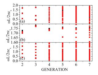
Figure 3. The evolutionary relationship of polaritonic band gaps with the Fibonacci generation  $l = 2 \sim 7$ ,  $\bar{L}_{M+} = 0.5\pi$  and  $\bar{L}_{M-} =$  $1.5\pi$  in frequency range of (a)  $\bar{\omega} = 0$ –2.0, (b)  $\bar{\omega} = 1.60$ –1.80 for the GFMS with m = 2 and (c)  $\bar{\omega} = 0$ –1.99 for the GFMS with m = 3. The other parameters are the same as Figure 2.
