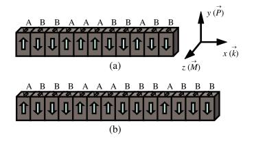
Figure 1. A schematic diagram of quasi-one-dimensional generalized Fibonacci multiferroic superlattices with the generation of l = 4 and the substitution index (a) m = 2 and (b) m = 3. Lattice displacement  $u_x$  and wavevector k are along x-axis, the magnetic field  $H_z$  and magnetization  $M_z$  are along  $\pm z$ -axis, the electric field  $E_y$  and polarization  $P_y$  are along  $\pm y$ -axis.
