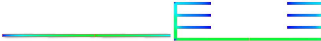
Figure 13. Distributed surface current along the proposed antenna structure compared to a conventional dipole antenna at 100 MHz centre frequency.
