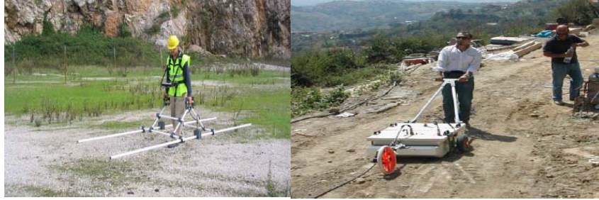
Figure 1. Archaeological GPR scanning with 100 MHz unshielded and shielded dipole antenna [7].
