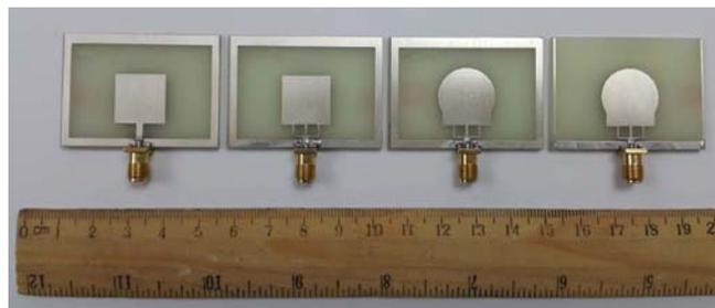
Figure 10. Photograph of the fabricated antennas.
