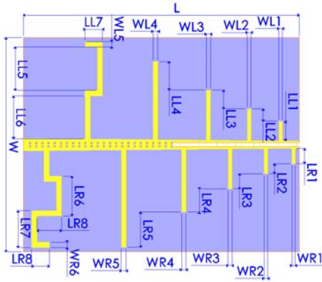
Figure 2. Geometry of the log-periodic radiating element.
