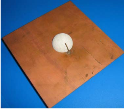
Figure 10. Fabricated antenna prototype for the arc-monopole coupled DRA.
