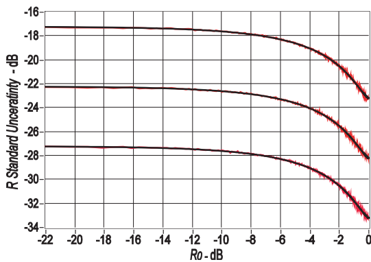
Figure 4. Numerical and analytical simulations of the standard uncertainty of R . The black traces are analytically simulated, whereas the red traces are numerically simulated. IL_{e,0} = -30 dB; IL_{e,0}/IL_{a,0} = 6 dB; IL_{a,S,0} changes from -35.98 dB to -30 dB, so that R_0 changes consequentially. For the upper trace, N = 10^4 ; for the middle trace, N = 10^5 ; for the lower trace, N = 10^6 . For the numerically simulated traces, T = 10^4 .
