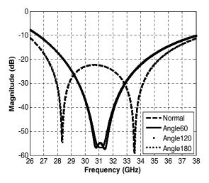
**Figure 7.** *X*-polarized wave reflected magnitude suppression.
