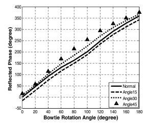
Figure 9. Reflected phase for different incidence angles vs bowtie rotation at 30 GHz.
