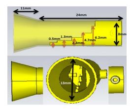
Figure 12. Ka-band CP feed horn.
