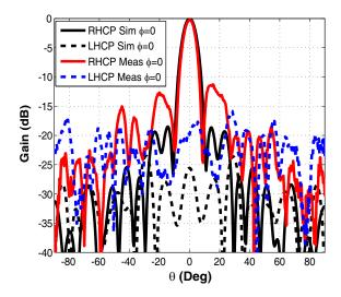
Figure 19. Simulated and measured RHCP and LHCP radiation patterns in XZ plane at 30 GHz.
