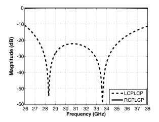
Figure 3. Copolar and cross polar components versus frequency.
