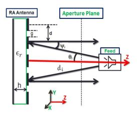
Figure 1. RA antenna basic structure.
