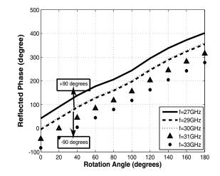
Figure 10. Bandwidth analysis for RA unit cell.
