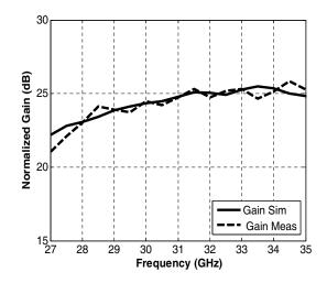
Figure 18. Simulated and measured gain curves.
