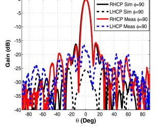
Figure 20. Simulated and measured RHCP and LHCP radiation patterns in YZ plane at 30 GHz.
