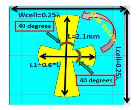
Figure 2. RA unit cell of the crossed bowtie.
