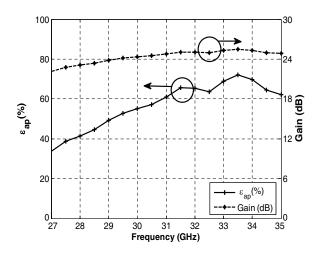
Figure 17. Gain variation with frequency of simulated RA.
