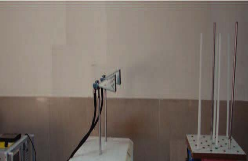
Figure 11. View of the experiment setup with antennas and targets.
