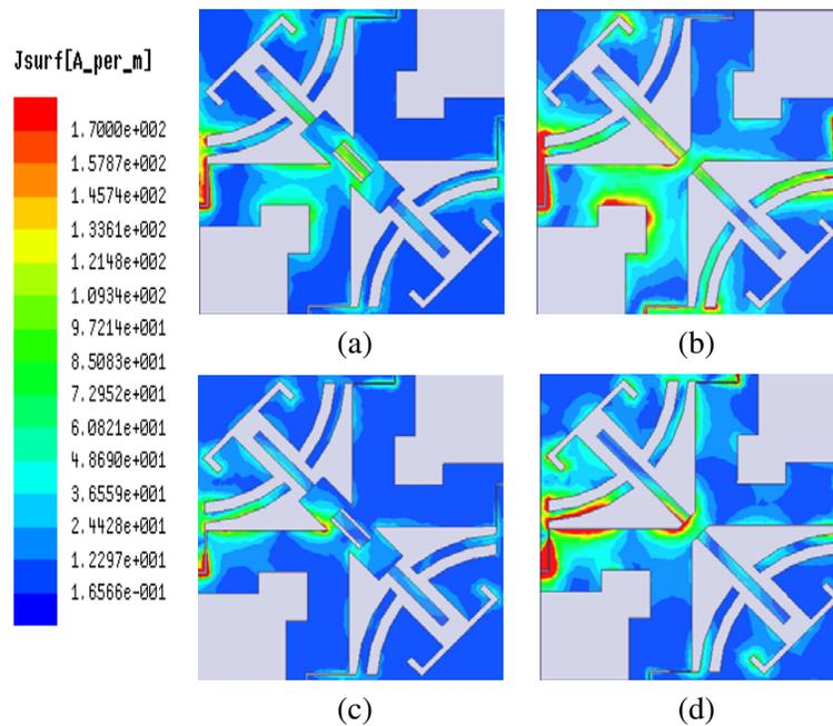
**Figure 3.** Simulated surface current distribution of the proposed antenna. (a) With the stub at 4.7 GHz. (b) Without the stub at 4.7 GHz. (c) With the stub at 10 GHz. (d) Without the stub at 10 GHz.
