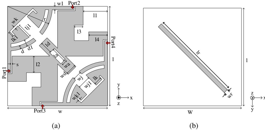
**Figure 1.** Configuration of the proposed ACS-fed UWB-MIMO antenna with shared radiators. (a) Top view. (b) Back view.
