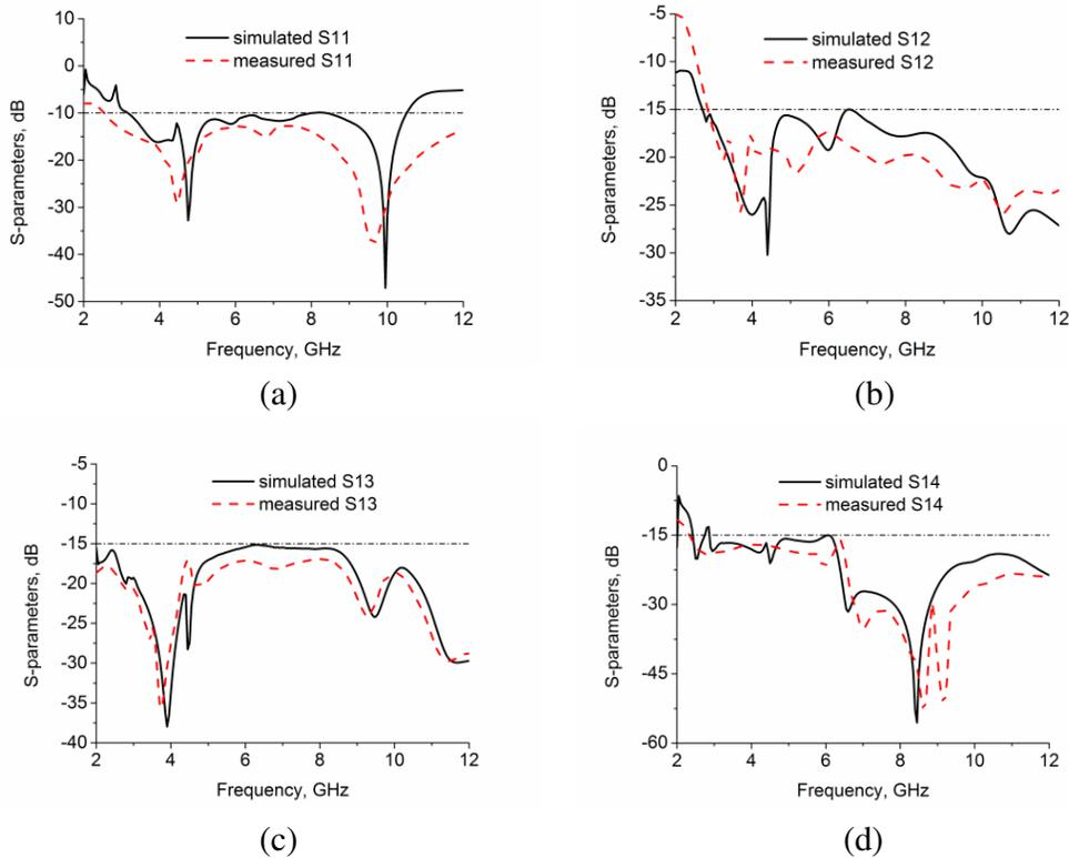
**Figure 8.** Simulated and measured  $S$ -parameters of the proposed antenna. (a)  $S_{11}$ . (b)  $S_{12}$ . (c)  $S_{13}$ . (d)  $S_{14}$ .
