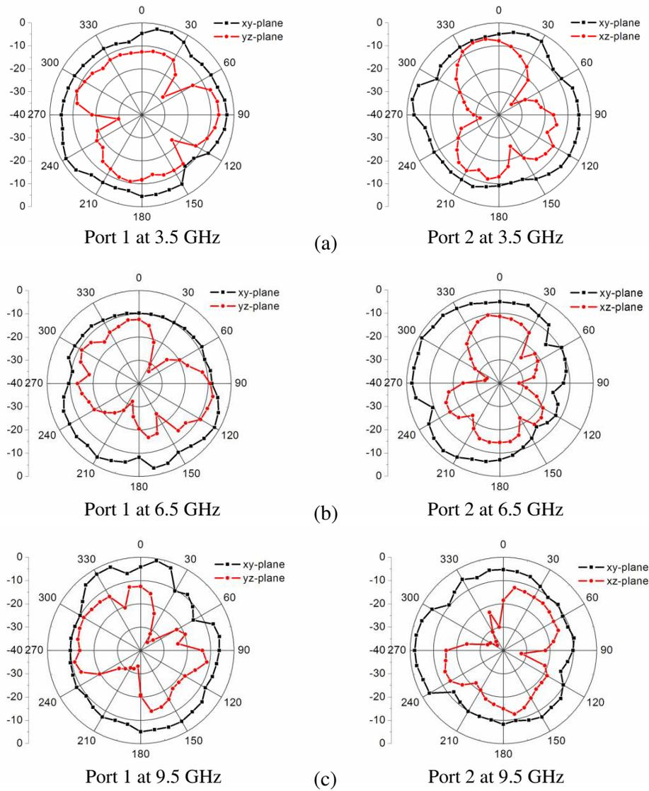
Figure 9. Measured radiation patterns of the proposed antenna. (a) 3.5 GHz. (b) 6.5 GHz. (c) 9.5 GHz.
