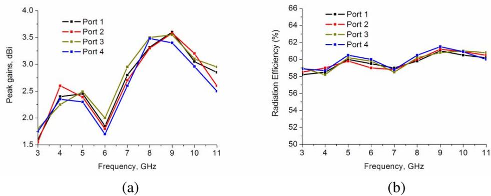
Figure 10. Measured peak gains and radiation efficiency of the proposed antenna. (a) Peak gains. (b) Radiation efficiency.
