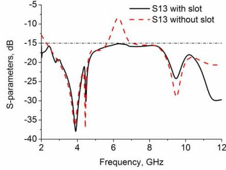
**Figure 4.** Simulated  $S_{13}$  of antenna when the rectangular slot varies.
