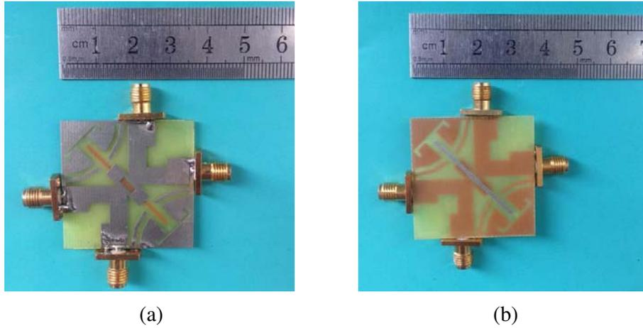
**Figure 7.** Photograph of the UWB-MIMO antenna. (a) Top view. (b) Back view.
