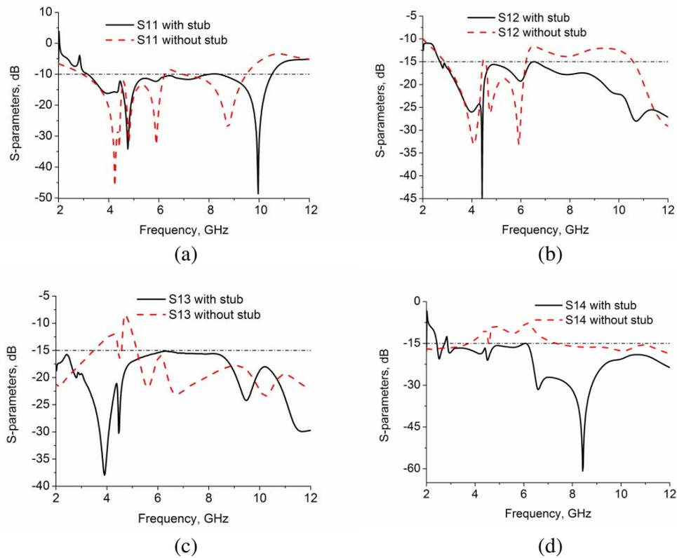
**Figure 2.** Simulated  $S$ -parameters of antenna when the stub varies. (a)  $S_{11}$ . (b)  $S_{12}$ . (c)  $S_{13}$ . (d)  $S_{14}$ .
