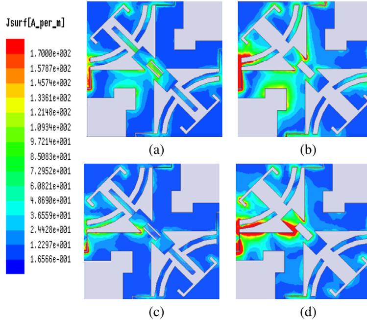
**Figure 6.** Simulated surface current distribution of the proposed antenna. (a) With the patch at 4.7 GHz. (b) Without the patch at 4.7 GHz. (c) With the patch at 10 GHz. (d) Without the patch at 10 GHz.
