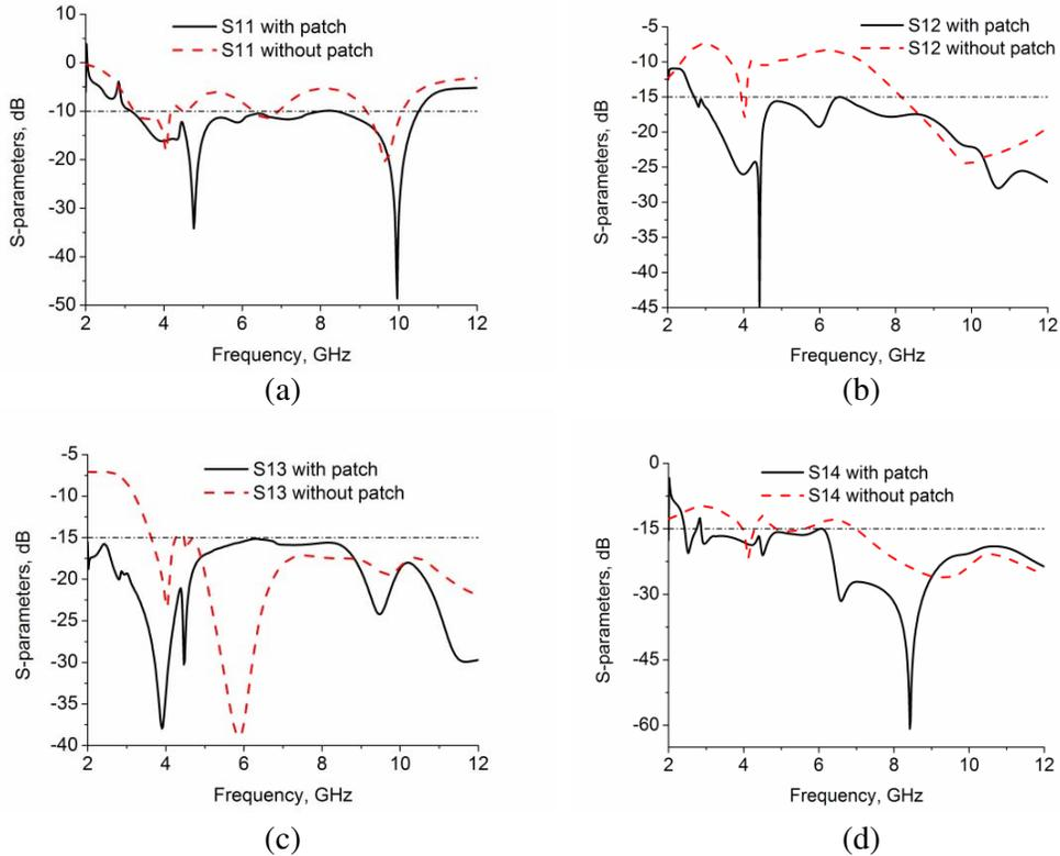
**Figure 5.** Simulated  $S$ -parameters of antenna when the patch varies. (a)  $S_{11}$ . (b)  $S_{12}$ . (c)  $S_{13}$ . (d)  $S_{14}$ .
