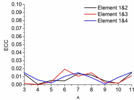
**Figure 11.** Measured envelop correlation coefficient.
