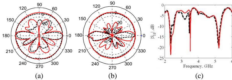
**Figure 4.** Simulated (solid) and measured (dashed) radiation pattern of the dual band OMA. (a) Radiation pattern at 2.45 GHz. (b) Radiation pattern at 5.2 GHz (inner:  $xy$  plane; outer:  $xz$ -plane). (c)  $|S_{11}|$ .
