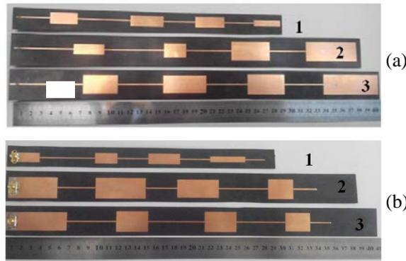
**Figure 5.** Photograph of the fabricated antennas. (a) Top view. (b) Bottom view (1: dual band, 2: wideband, 3: high gain).
