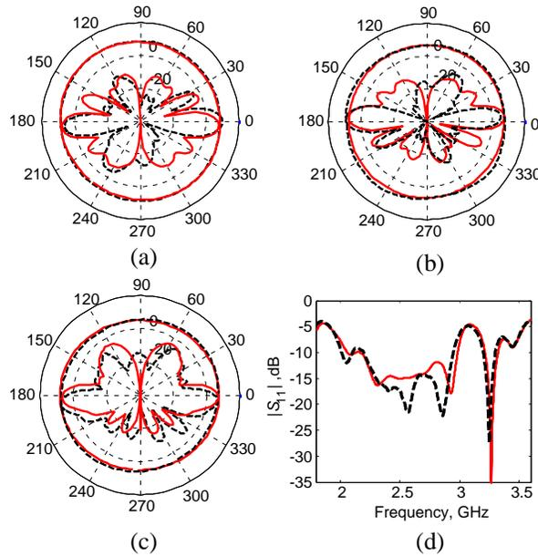
**Figure 2.** Simulated (solid) and measured (dashed) radiation pattern of the wideband OMA. (a) 2.25 GHz. (b) 2.45 GHz. (c) 2.65 GHz. (d)  $|S_{11}|$  (inner:  $xy$ -plane; outer:  $xz$ -plane).
