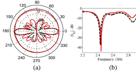
**Figure 3.** Simulated (solid) and measured (dashed) radiation pattern of the high gain OMA. (a) Radiation pattern at 2.45 GHz (inner:  $xy$  plane; outer:  $xz$ -plane). (b)  $|S_{11}|$ .
