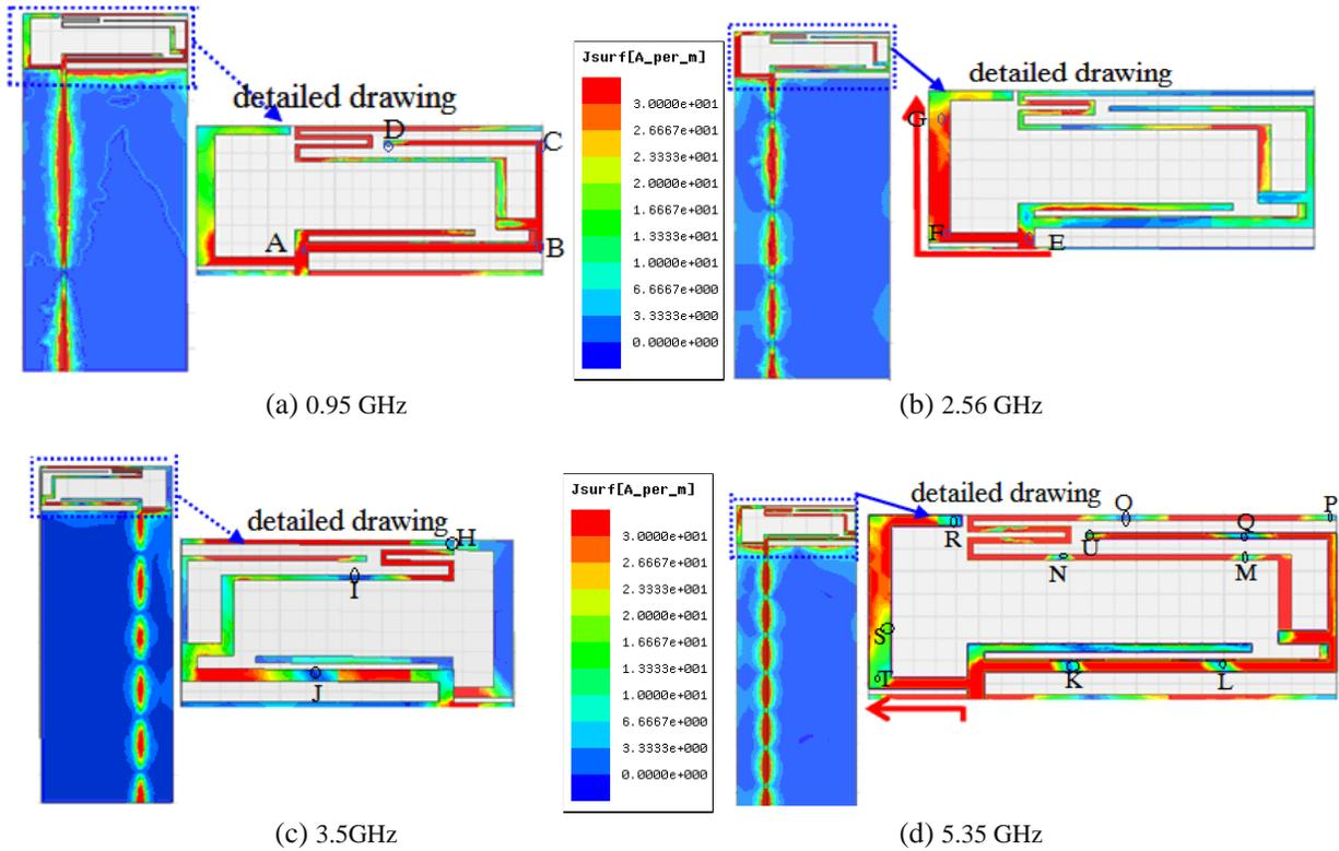
Figure 6. Current distributions at 800 MHz 2.56/3.5/5.35 GHz.
