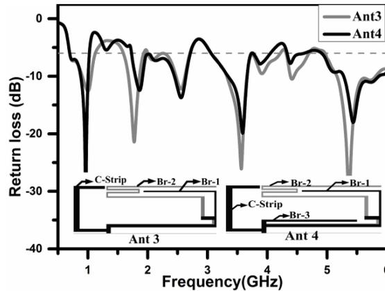
Figure 5. Simulated return loss for Ant3 and Ant4.
