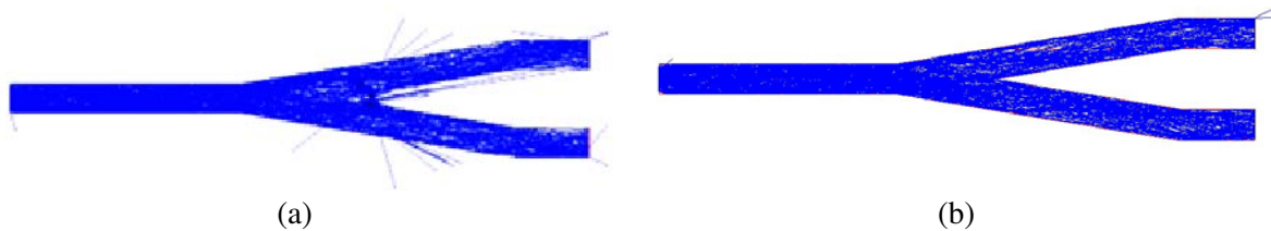
Figure 3. 2D ray tracing diagram for 1 \times 2 Y-branch POF coupler. (a) Design 1. (b) Design 2.
