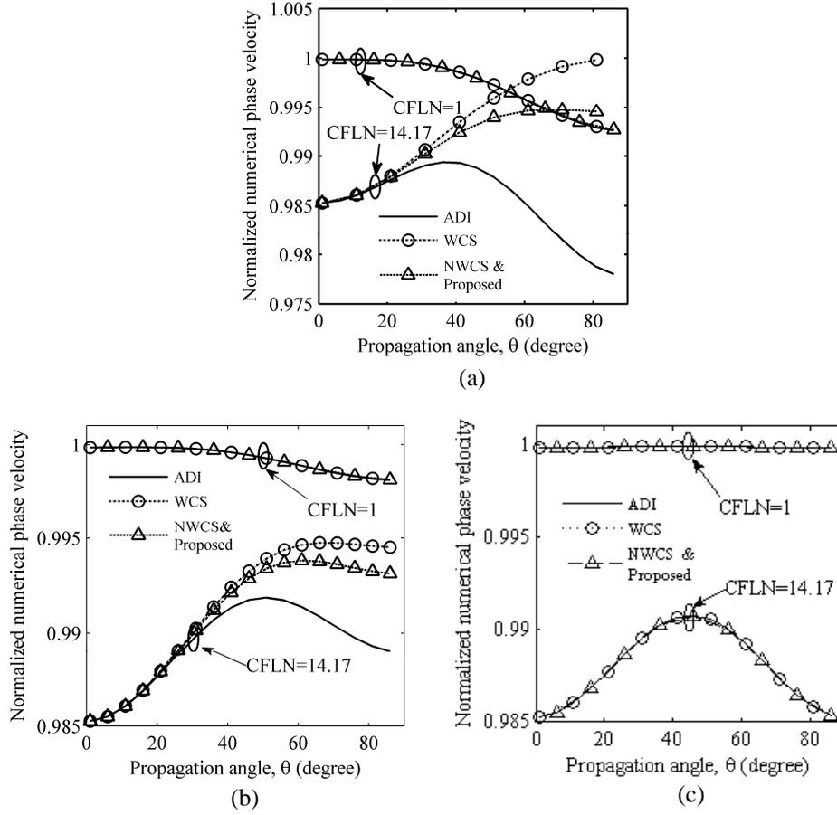
**Figure 1.** Normalized phase velocities versus propagation angle  $\theta$  for different methods: (a)  $\varphi = 0^\circ$ , (b)  $\varphi = 45^\circ$ , and (c)  $\varphi = 90^\circ$ .
