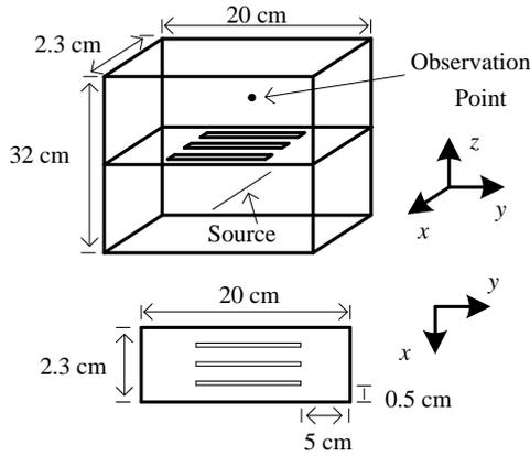
**Figure 3.** Enclosure with a thin metal plate.
