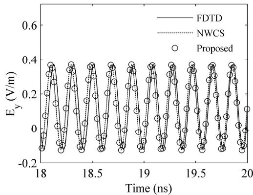
**Figure 2.** Time domain waveforms of  $E_y$ .
