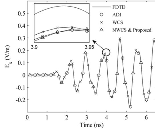
**Figure 4.** Time domain waveforms of  $E_x$  excited by Gaussian pulse.
