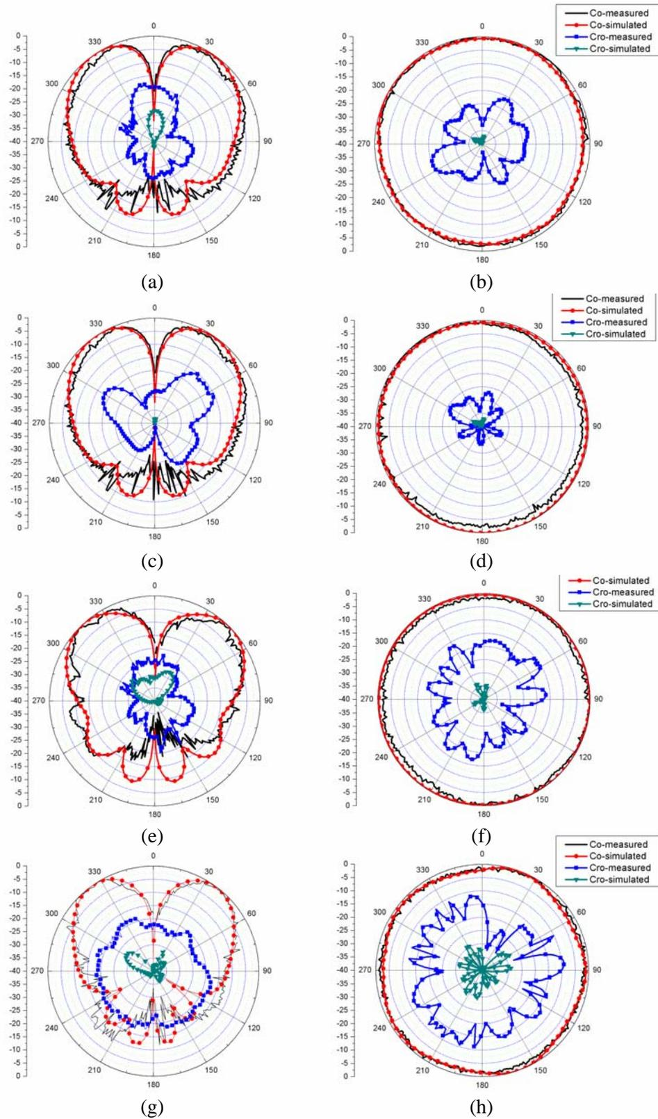
**Figure 8.** Elevation plane radiation patterns for the fabricated antenna at: (a) 4.42 GHz, (c) 4.67 GHz, and (e) 5.25 GHz, (g) 6.42 GHz. Azimuth plane radiation patterns at: (b) 4.42 GHz, (d) 4.67 GHz and (f) 5.25 GHz, (h) 6.42 GHz.
