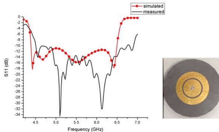
Figure 7. Reflection coefficients for the fabricated antenna and the photograph are shown in the inset.
