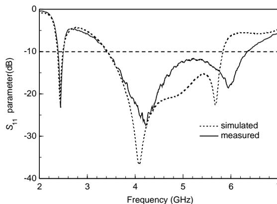
**Figure 4.** Measured and simulated  $S_{11}$  parameters against frequency for the proposed dual-band antenna.
