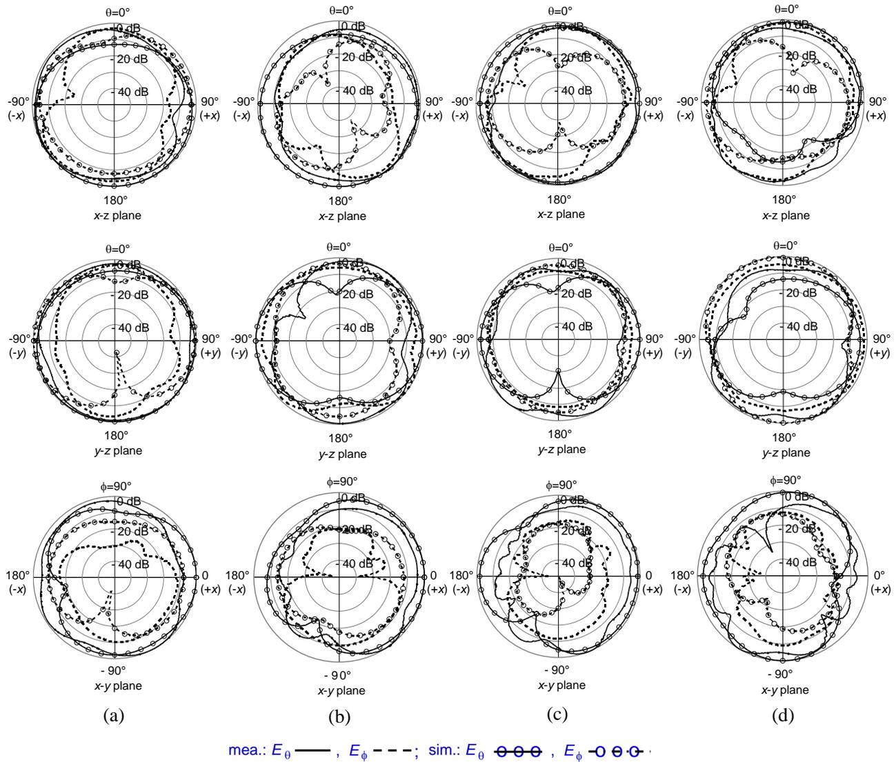
**Figure 5.** Normalized radiation patterns obtained from simulation and measurement for proposed antenna at (a) 2.45 GHz, (b) 3.5 GHz, (c) 5.25 GHz, and (d) 5.75 GHz.
