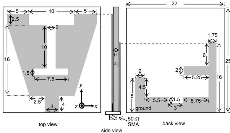
**Figure 1.** Configuration of proposed dual-band planar slotted patch antenna for WLAN/WiMAX operations (dim. in mm).
