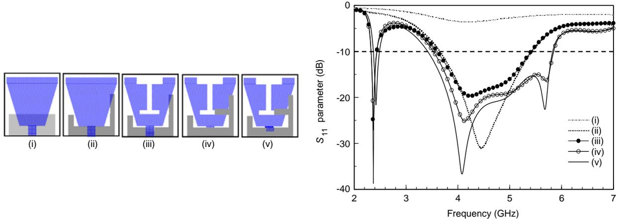
**Figure 2.** Simulated  $S_{11}$  parameters of the proposed antenna with different structures.
