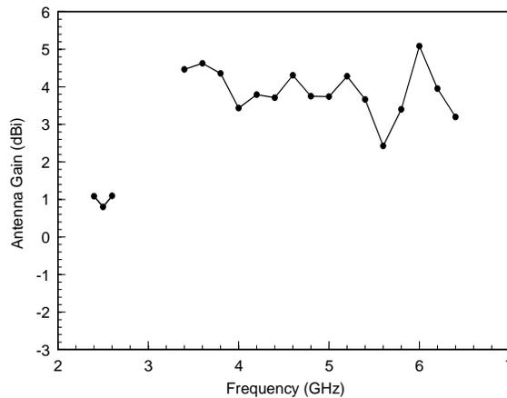
**Figure 6.** Measured peak antenna gains across the lower and upper bands for the proposed antenna.
