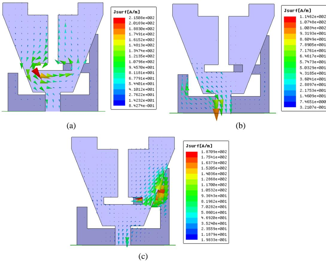
**Figure 3.** Simulated surface current distributions for the proposed antenna studied in Figure 1: (a)  $f = 2.42$  GHz; (b)  $f = 4.08$  GHz; (c)  $f = 5.68$  GHz.
