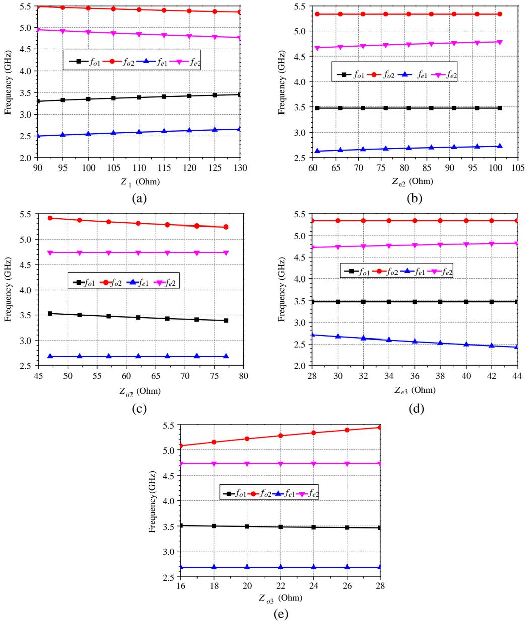
**Figure 4.** The influence of characteristic impedances on resonant frequencies under (a)  $Z_1$ , (b)  $Z_{e2}$ , (c)  $Z_{o2}$ , (d)  $Z_{e3}$ , and (e)  $Z_{o3}$ .
