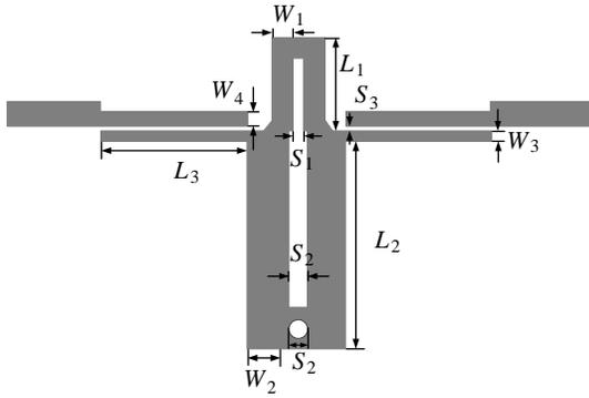
**Figure 2.** Layout of the proposed filter.
