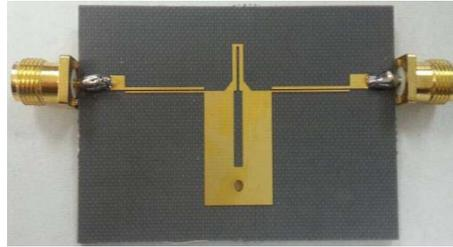
Figure 5. Photograph of the fabricated filter.
