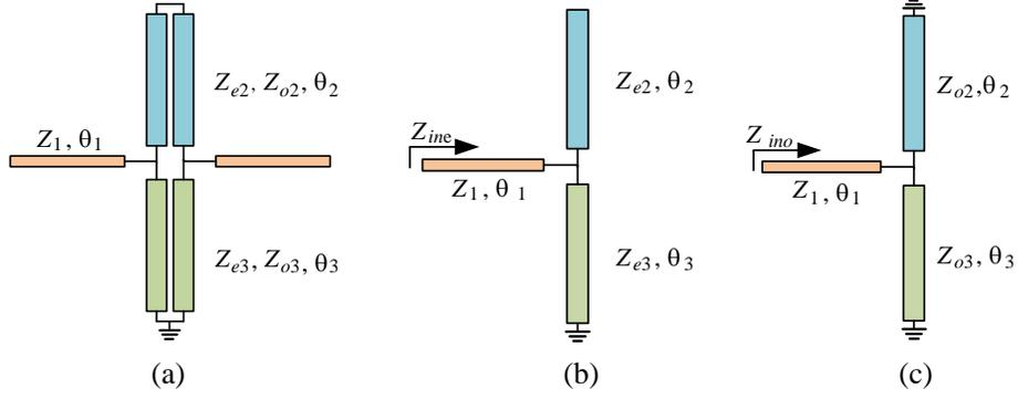
**Figure 1.** (a) Circuit configuration of the modified resonator. (b) Even-mode equivalent circuit. (c) Odd-mode equivalent circuit.
