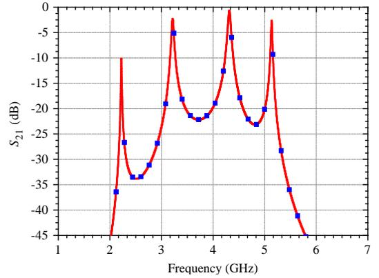
**Figure 3.** Full-wave simulated result of the proposed resonator.
