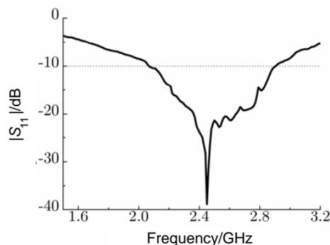
**Figure 5.**  $|S_{11}|$  of the rectifying circuit simulated by ADS.
