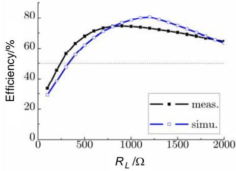
**Figure 7.** Simulated and measured efficiency vs. load.
