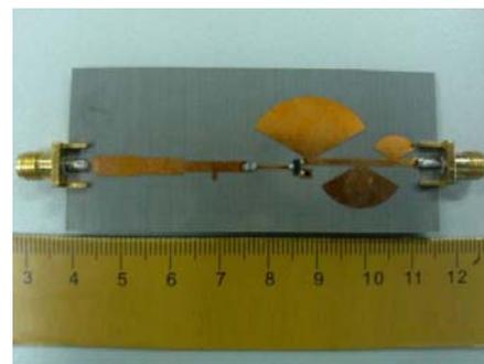
**Figure 6.** Photograph of the fabricated rectifying circuit.
