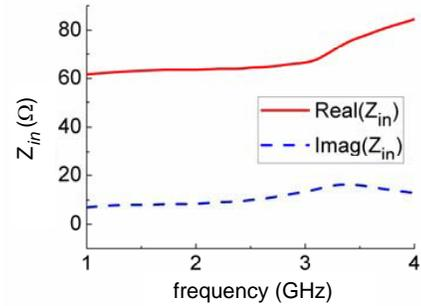
**Figure 2.** Input impedance  $Z_{in}$  vs. frequency simulated by ADS.
