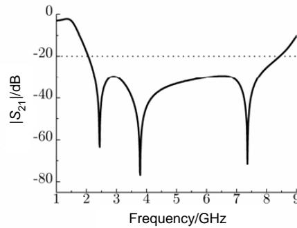
**Figure 4.**  $|S_{21}|$  of the dc-pass filter simulated by ADS.
