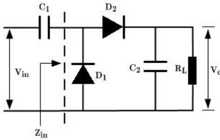
**Figure 1.** Basic model of the voltage doubling circuit.
