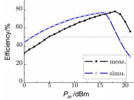
**Figure 8.** Simulated and measured efficiency vs. input power.
