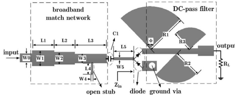
**Figure 3.** Layout of the designed voltage doubling rectifying circuit.
