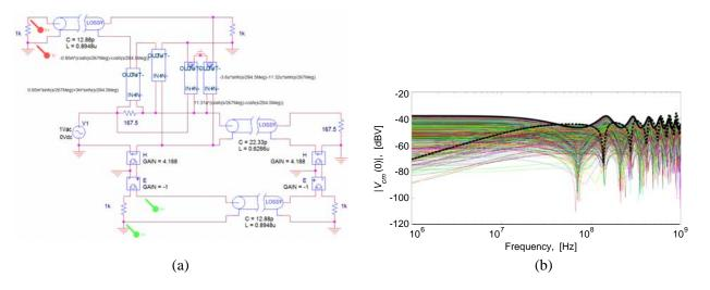
Figure 12. Inhomogeneous medium: (a) SPICE schematic of the unbalanced DL excited by a DM source. (b) SPICE predictions (black curves) vs 1000 repeated simulations obtained by exact solution of MTL equations (left TL end).
