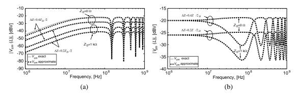
Figure 6. CM voltages due to termination imbalance: proposed model (dotted curves) vs exact MTL solution (grey-solid curves). Influence of the ground impedance (i.e.,  $Z_G = 0 \Omega$ ,  $1 k\Omega$ ) for (a)  $\Delta Z = \Delta Z_L = \Delta Z_R$ , (b)  $\Delta Z = \Delta Z_L = -\Delta Z_R$ .
