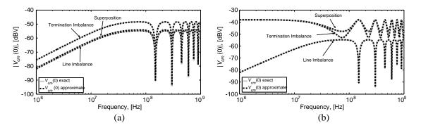
Figure 9. CM voltages obtained by superposition of the contributions due to line and termination imbalance  $(Z_G = 1 \text{ k}\Omega)$ : (a)  $\Delta Z_L = \Delta Z_R$ ; and (b)  $\Delta Z_L = -\Delta Z_R$ .
