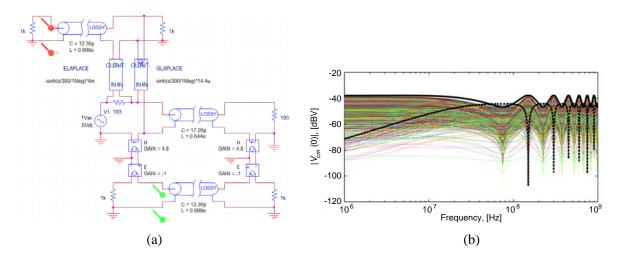
**Figure 11.** Implementation in SPICE: (a) schematic of the unbalanced DL excited by a DM source. (b) SPICE predictions (black curves) vs 1000 repeated simulations obtained by exact solution of MTL equations (left TL end).
