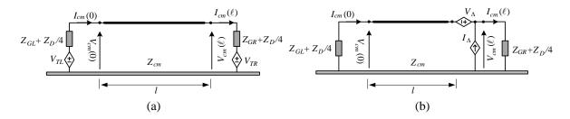
Figure 5. CM circuits accounting for DM-to-CM conversion due to (a) line and (b) termination imbalance.
