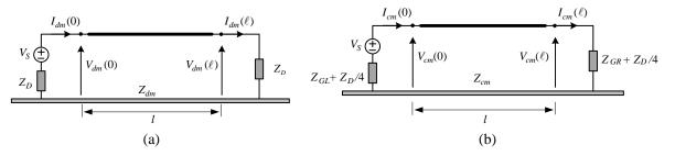
**Figure 3.** Approximate (a) DM and (b) CM circuits obtained under the assumption of weak unbalance for (a) DM and (b) CM excitation of the DL circuit in Figure 1.
