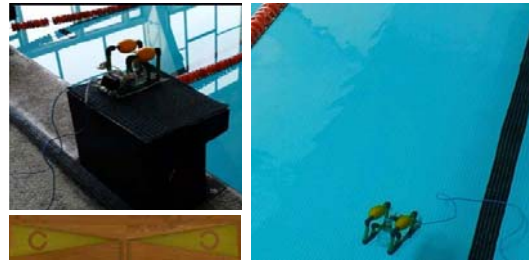
Figure 7. The hydrobot used for performing tests. Identical antennas were placed at the lower tubes.
