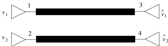
Figure 3. Two parallel microstrip lines with consistent parameters.
