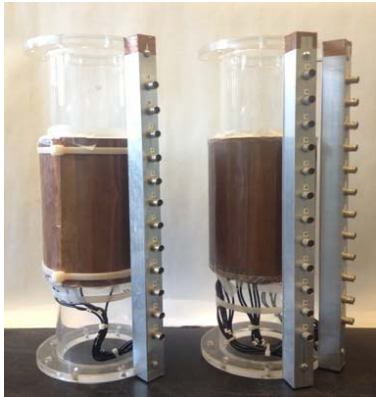
Figure 2. Two ECVT sensors of 12 and 24 plates covering the same imaging volume.
