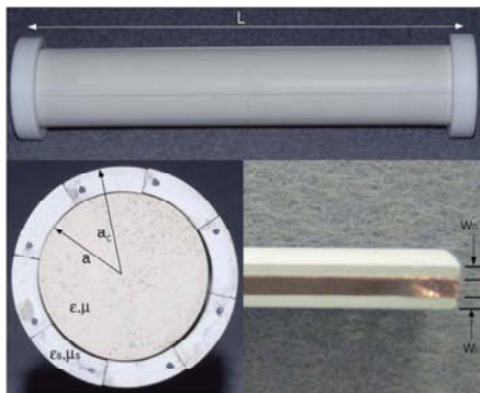
Figure 13. Experimental validation of plasmonic cloaking in free-space: cloaked cylinder. ©2012 IOP Publishing. Reprinted with permission [155].
