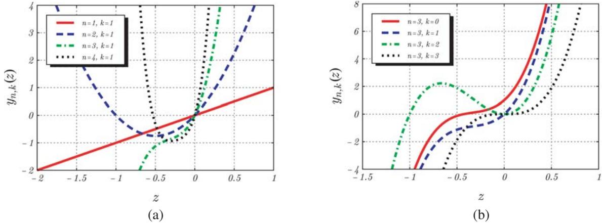
**Figure 4.** Distribution of the incomplete Bessel polynomial  $y_{n,k}(z)$  for different orders  $n$  (a) and  $k$  (b).
