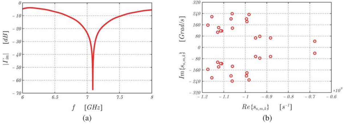
**Figure 6.** Frequency-domain behavior of the input reflection coefficient (a) and distribution of the resonant poles, (b) featured by the hemispherical dielectric lens antenna shown in Fig. 1.
