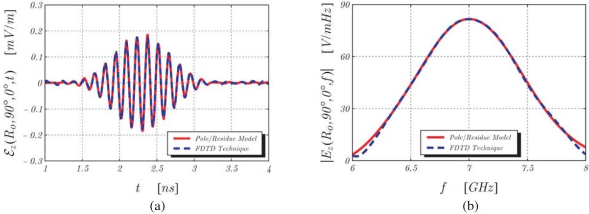
**Figure 7.** Transient (a) and frequency-domain, (b) behavior of the co-polarized electric field component excited by the hemispherical dielectric lens antenna shown in Fig. 1 at a distance  $R_O = 6.0$  cm from the ground plane along the boresight direction ( $x$ -axis in the adopted coordinate system).
