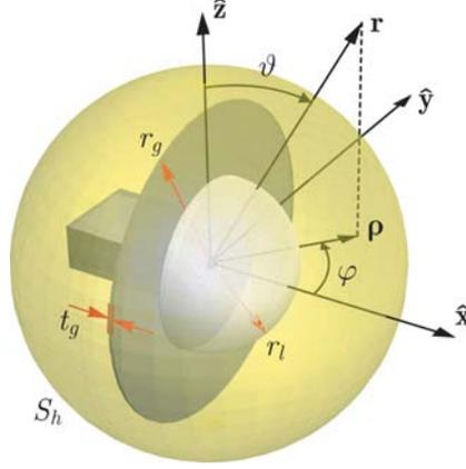
**Figure 1.** Dielectric lens antenna enclosed by a spherical Huygens surface  $S_h$ . The coordinate system adopted to express the electromagnetic field quantities is also shown.
