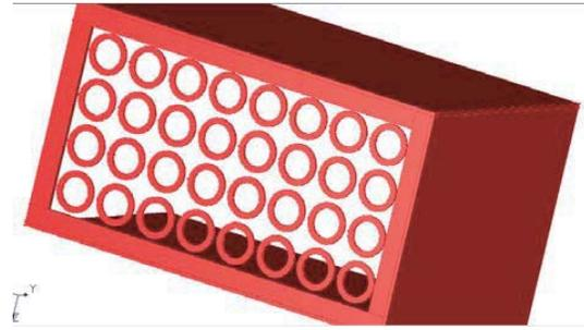
**Figure 6.** Microwave enclosures with ring cross FSS wall.
