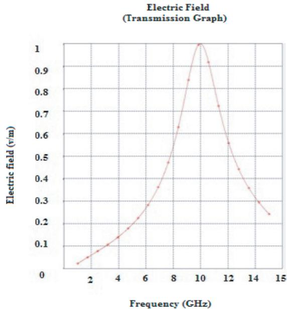
**Figure 8.** Response curve between electric field vs. frequency.
