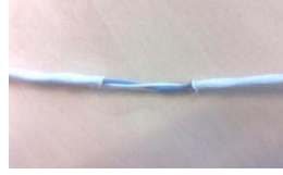
Figure 2. AWG24 twisted pair with a soft defect.
