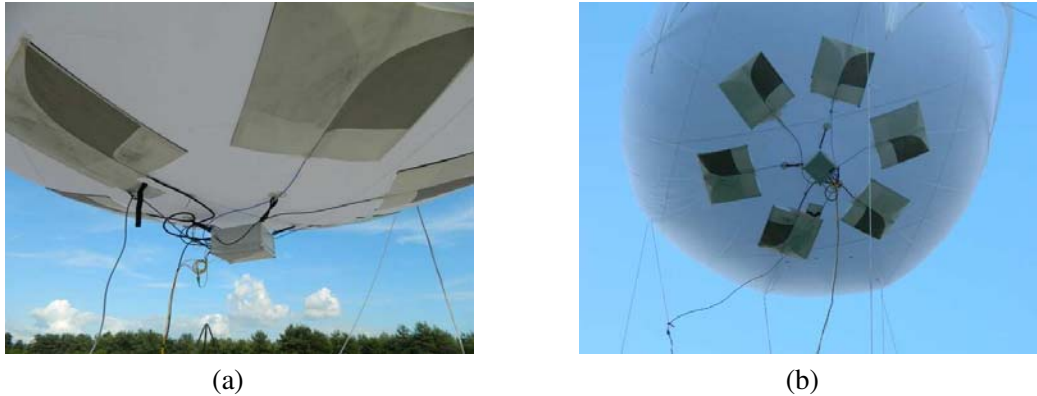
Figure A1. Six identical antennas under a gas balloon during a test manipulation.
