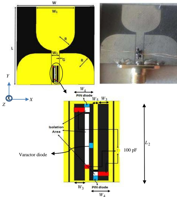
**Figure 1.** Photograph of the fabricated antenna with resonance cell, PIN diodes and varactor diode.
