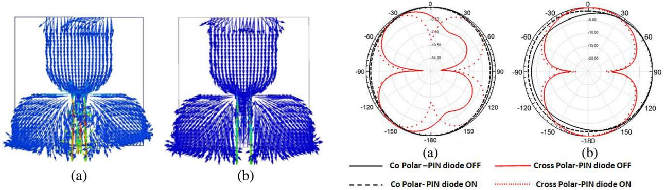
**Figure 3.** Electric field distribution at 5.8 GHz with two PIN diodes. (a) PIN diodes OFF state. (b) PIN diodes ON.
