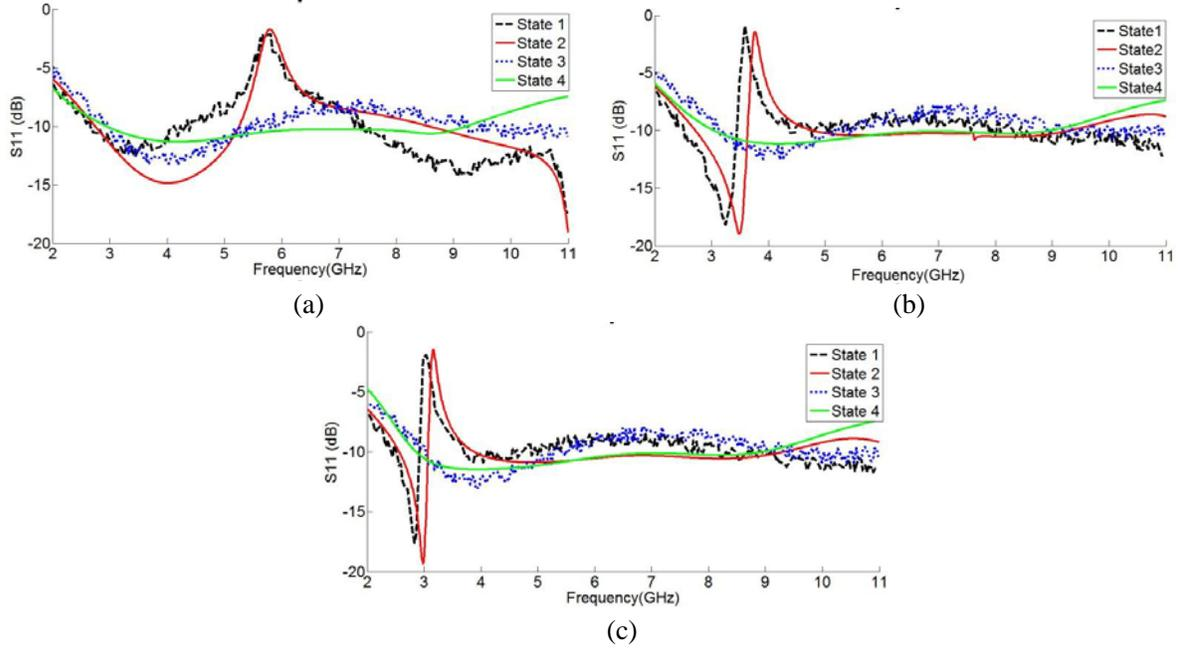
**Figure 2.** Measured and simulated return loss of the reconfigurable antenna (according to the Table 1).
