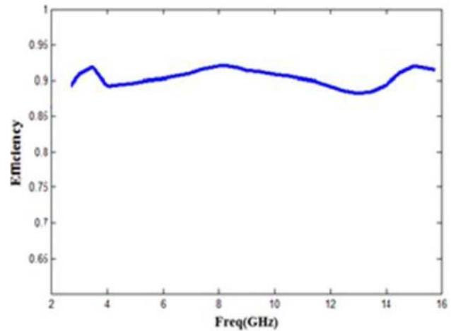
**Figure 6.** Radiation efficiency of the antenna.
