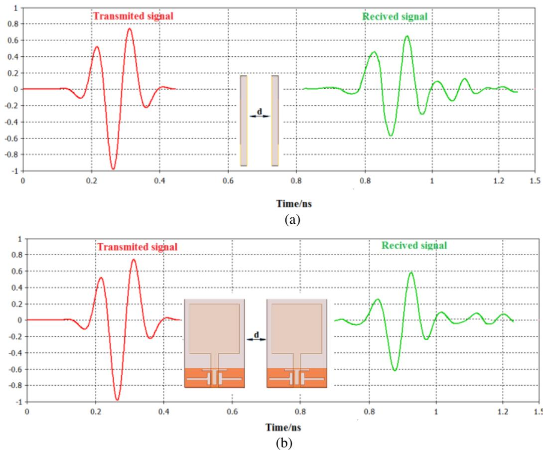
**Figure 11.** Transmitted and received signals, (a) face to face and (b) side by side.
