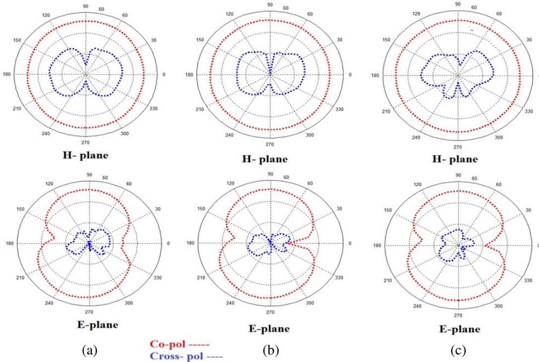
**Figure 8.** Measured radiation patterns of the proposed antenna, (a) 4.5 GHz, (b) 10 GHz, and (c) 13.5 GHz.
