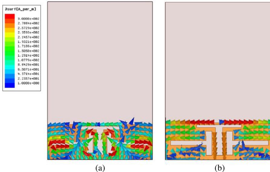
**Figure 7.** Current distributions in the ground plane for proposed antenna at the additional resonances frequencies, (a) 12.1 GHz, (b) 15.3 GHz.
