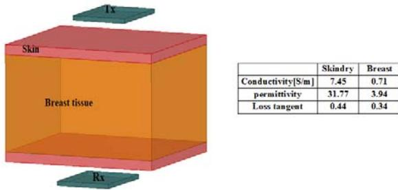
**Figure 9.** Configuration of the compressed breast model with two antennas.
