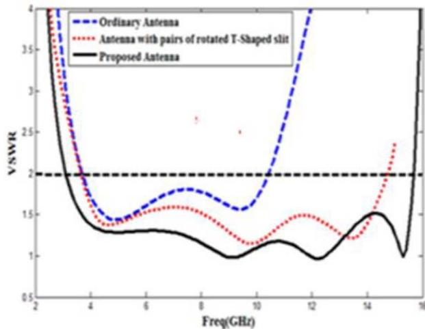
**Figure 3.** Simulated VSWR characteristics of the various structures shown in Figure 2.
