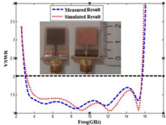
**Figure 4.** Measured and simulated VSWR of the antenna.
