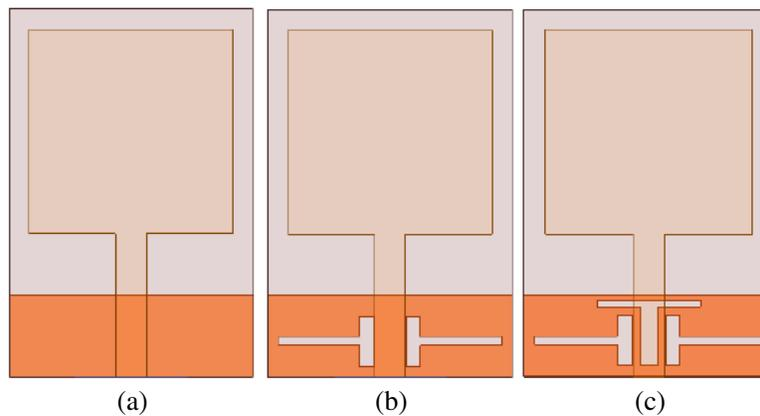
**Figure 2.** The step by step development of the antenna used for multi resonance performance simulation.
