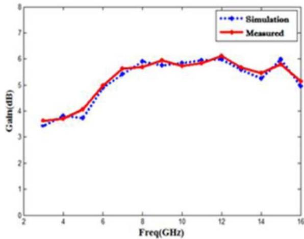
**Figure 5.** Measured and simulated gains of the antenna.
