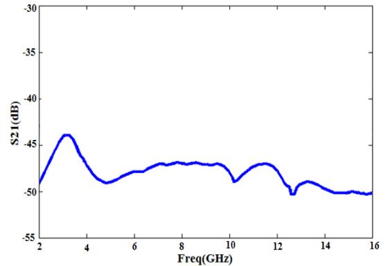
**Figure 10.** The transmission parameter  $S_{21}$  of the antenna.
