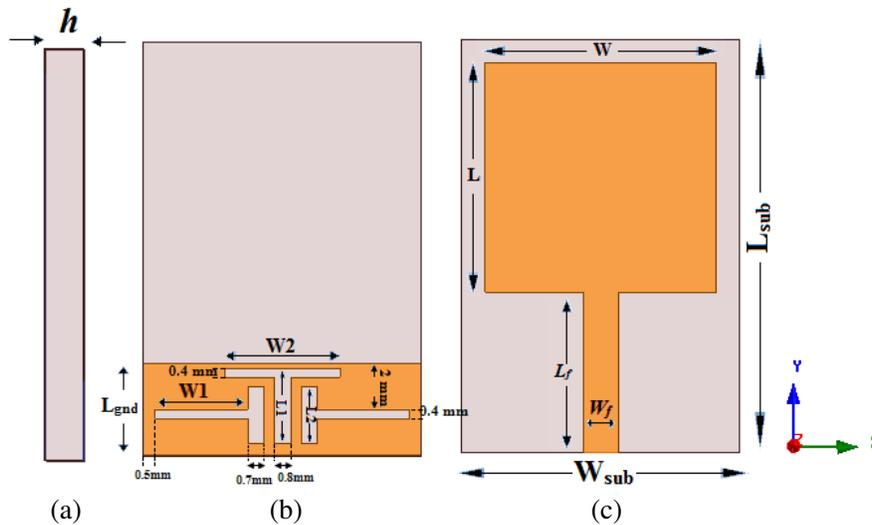
**Figure 1.** The configuration of the proposed, (a) side view, (b) top layer, and (c) bottom layer.
