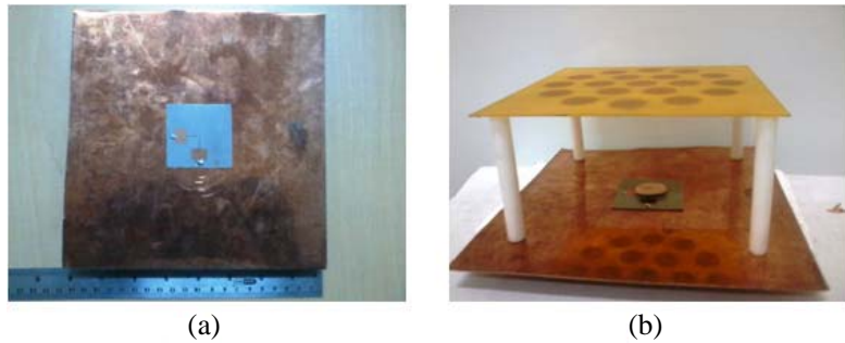
Figure 7. Fabricated 1B19T dual polarized space-fed antenna array, (a) bottom ground plane with dual feeds and (b) integrated antenna array with top parasitic elements.
