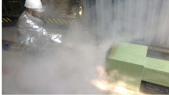
**Figure 3.** Picture of one of the performed experiment. A stream of water is poured onto the sheet metal, measured by the radiometer.
