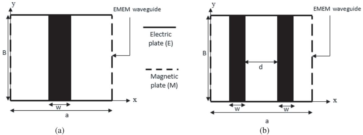
**Figure 1.** Studied structures (a) Structure 1: one micro-strip in a rectangular electric magnetic electric magnetic (EMEM) waveguide. (b) Structure 2: two micro-strips in a rectangular (EMEM) waveguide.  $a = 20$  mm,  $B = 9$  mm,  $w = 1$  mm and  $d = 5$  mm.
