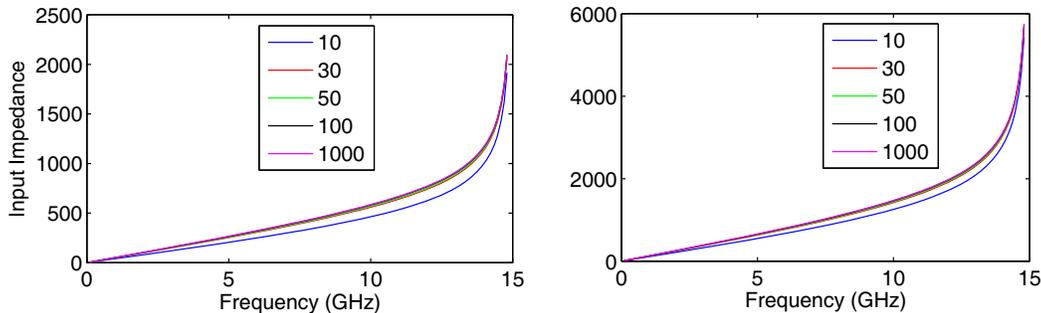
**Figure 4.** Study of input impedances convergence. Input impedances versus frequency for various used modal basis functions number. (a) Structure 1 (only one microstrip). (b) Structure 2 (two microstrips).
