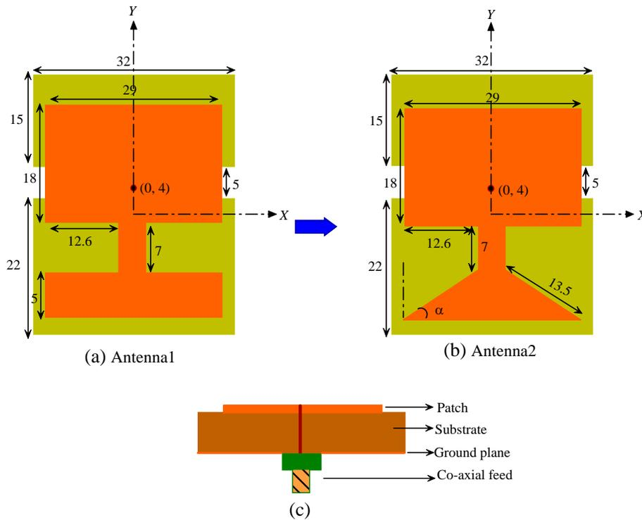
**Figure 1.** Geometrical configurations of the proposed antennas, (a), (b) top view and (c) side view (units are in mm).
