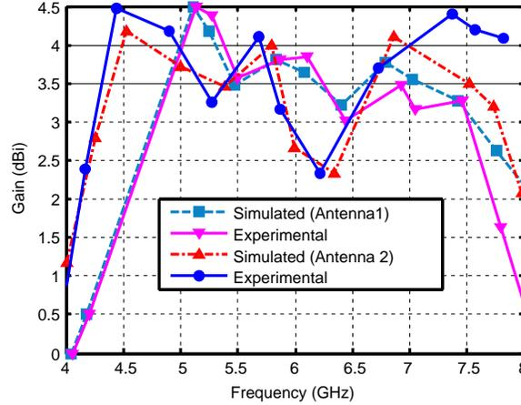
Figure 8. Gain versus frequency plot of proposed Antenna1 and Antenna2.
