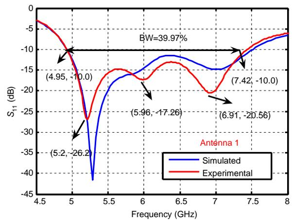
**Figure 5.** Plot of reflection coefficient versus frequency for proposed Antenna1.
