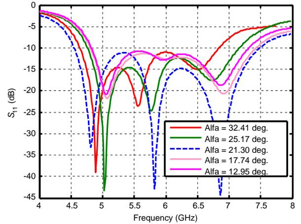
**Figure 7.** Variation of the reflection coefficient versus frequency at different inclination angles.
