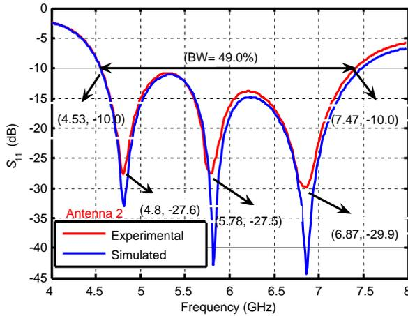
**Figure 6.** Plot of reflection coefficient versus frequency for proposed Antenna2.
