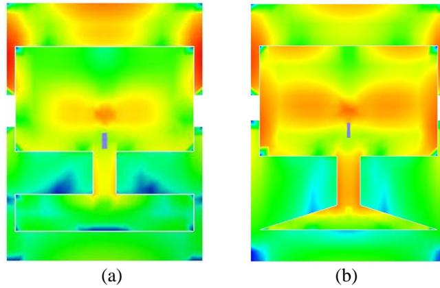
**Figure 3.** Current distribution of the proposed (a) Antenna1 at center frequency  $f_r = 6.20$  GHz and (b) Antenna2 at center frequency  $f_r = 6.0$  GHz.
