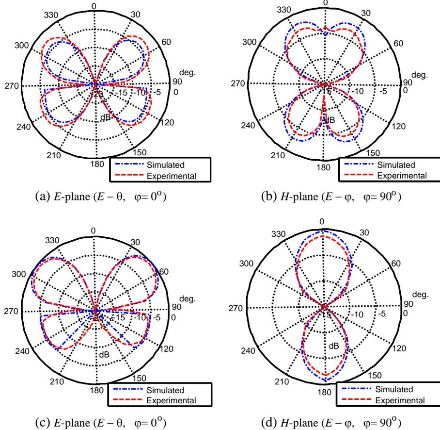
Figure 9. Radiation-field patterns of  $E$  and  $H$  plane for (a), (b) rectangular base desktop shaped patch antenna (Antenna1) at 6.20 GHz and (c), (d) triangular base desktop shaped patch antenna (Antenna2) at 6.0 GHz.
