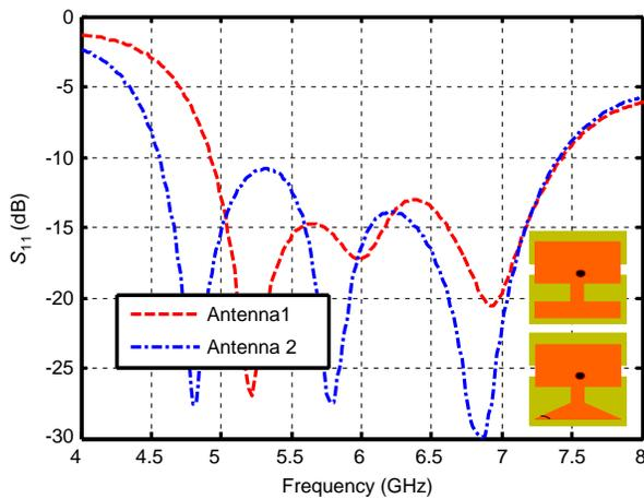
**Figure 4.** Comparative plot of reflection coefficient versus frequency for proposed Antenna1 and Antenna2.
