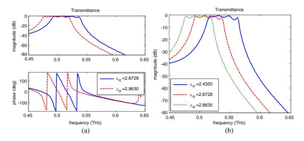
Figure 9. Transmittance of metallic grating with 3 equispaced cuts tuned within (a) half the range and (b) the whole range of E7 permittivity values ( $a = 60 \,\mu\text{m}$ ,  $p = 300 \,\mu\text{m}$ ,  $w = 1500 \,\mu\text{m}$ ,  $d = 70 \,\mu\text{m}$ ,  $l = 50 \,\mu\text{m}$ ,  $\sigma = 5.86 \times 10^7$ ).
