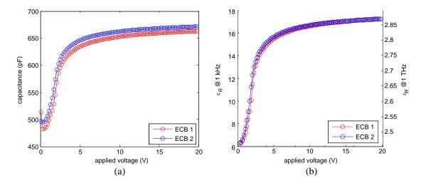
**Figure 2.** (a) Capacitance variation versus 1 kHz applied voltage for Brass + E7 ECB cells. (b) Estimated permittivity variation with voltage at 1 kHz and 1 THz.
