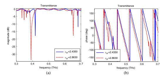
Figure 12. (a) Magnitude and (b) phase of the transmission coefficient of the dielectric grating with non-continuous electrodes ( $a = 60 \,\mu\text{m}, p = 300 \,\mu\text{m}, w = 1500 \,\mu\text{m}, \sigma = 5.86 \times 10^7, \varepsilon_{R\_dielectric} = 2.1000$ ).
