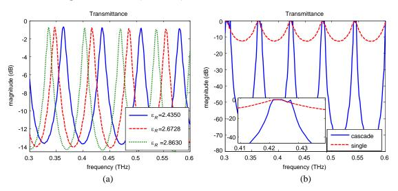
Figure 3. (a) Transmittance of metallic grating with the variation of LC permittivity. (b) Transmittance of a cascade of 4 metallic gratings with 130 µm separation (a = 60 µm, p = 300 µm, w = 1500 µm,  $\varepsilon_R = 2.6728$ ,  $\sigma = 5.86 \times 10^7$ ).
