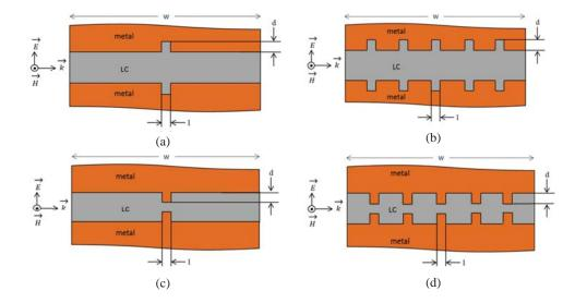
Figure 7. Metallic grating with (a) one and (b) multiple cuts and with (c) one and (d) multiple obstacles.
