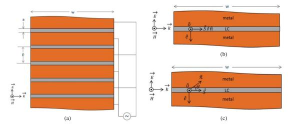
**Figure 1.** (a) Metallic grating geometry and propagation. (b) Orientation of the LC director axis with no voltage applied. (c) Orientation of the LC director axis with voltage applied.
