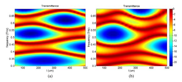
Figure 8. Transmittance of metallic grating with (a) one cut in the middle and (b) two cuts equispaced from each other and from the edges as a function of frequency and width of the cuts ( $a = 60 \,\mu\text{m}$ ,  $p = 300 \,\mu\text{m}$ ,  $w = 1500 \,\mu\text{m}$ ,  $d = 30 \,\mu\text{m}$ ,  $\varepsilon_R = 1$ ,  $\sigma = 10^{12}$ ).
