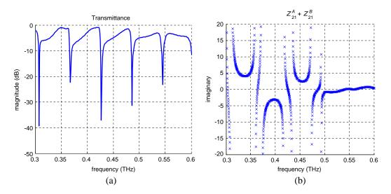
Figure 11. Transmittance of the dielectric grating with continuous electrodes and imaginary part of the sum of the two-port network impedances showing the zero-crossing  $(a = 60 \,\mu\text{m}, p = 300 \,\mu\text{m})$  $w = 1500 \ \mu\text{m}, \ \varepsilon_R = 2.6490, \ \sigma = 10^{12}, \ \varepsilon_{R-dielectric} = 2.1).$
