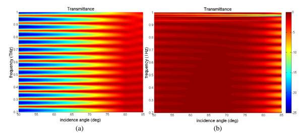
Figure 6. Transmittance with the variation of incident angle for (a) a grating with a small LC thickness and (b) a large LC thickness ( $a = 30 \,\mu\text{m}$  and  $100 \,\mu\text{m}$ ,  $p = 150 \,\mu\text{m}$ ,  $w = 1500 \,\mu\text{m}$ ,  $\varepsilon_R = 2.649$ ,  $\sigma = 5.86 \times 10^7$ ).
