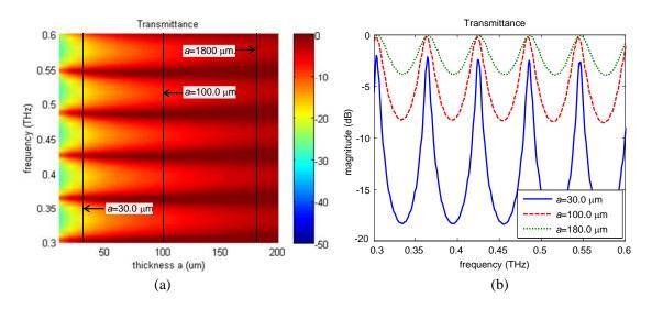
Figure 4. Transmittance of metallic grating with variating LC layer thickness ( $p = 300 \,\mu\text{m}$ ,  $w = 1500 \,\mu\text{m}$ ,  $\varepsilon_R = 2.649$ ,  $\sigma = 5.86 \times 10^7$ ).
